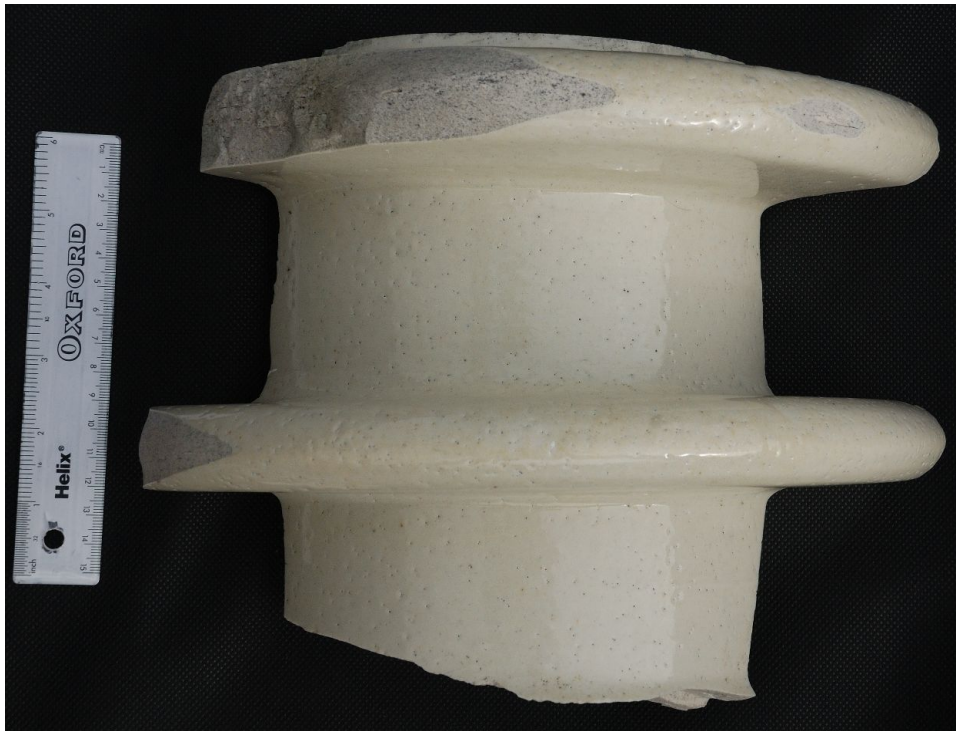
C15. A very large, cream-white glazed insulator found at a brake/winding base at the top of the incline for construction of the 1923 extension. This was one of the through-wall insulators seen in several photographs of the inductor ('ATI') houses; intact examples are still seen at the transmitter house. Connections were made to a metal plate with a conductor that ran within the insulator and thus passed through building walls. Its position at the top of the incline suggests it was one of the lower inductor house insulators, probably discarded as of no further use after being transported with scrap metal by rail truck to the summit of Cefn Du. Numerous fragments of the same type of insulator, but with a whiter glaze, were found buried in a nearby boggy pool (marked in context, below, at 53.123069° -4.171382°).
