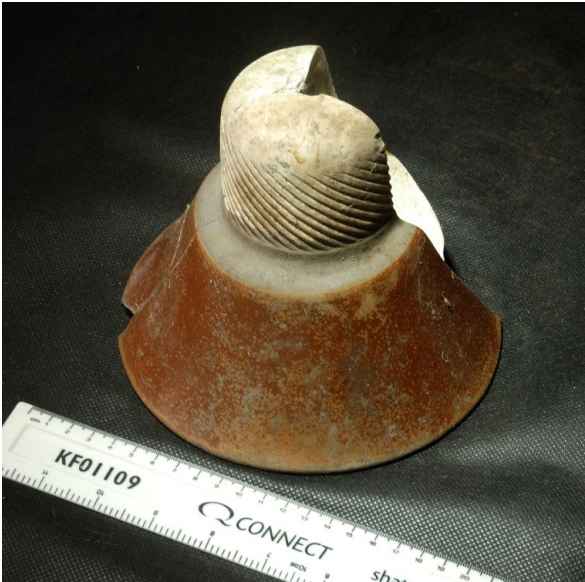
C25 , above: Part of the P.5656, nested 'pin' insulator with a central threaded section containing cementing and a lead (metal) collar.
