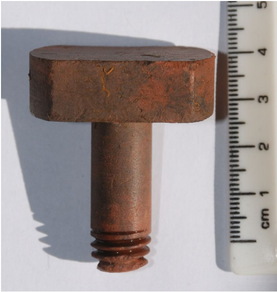
D7, left: found near the angled turn at the northern end of the double ATI, a ceramic, single-piece threaded bolt. The inductor ring above is seen to have such a handle on its bolts, but it is not entirely clear if they are exactly the same type.
