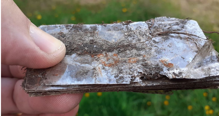
C28. Part of a mica sheet capacitor, probably a mica-silver type, as there are no interleaved copper sheets as in mica capacitors before this period. Length = 3", width = 1½".
