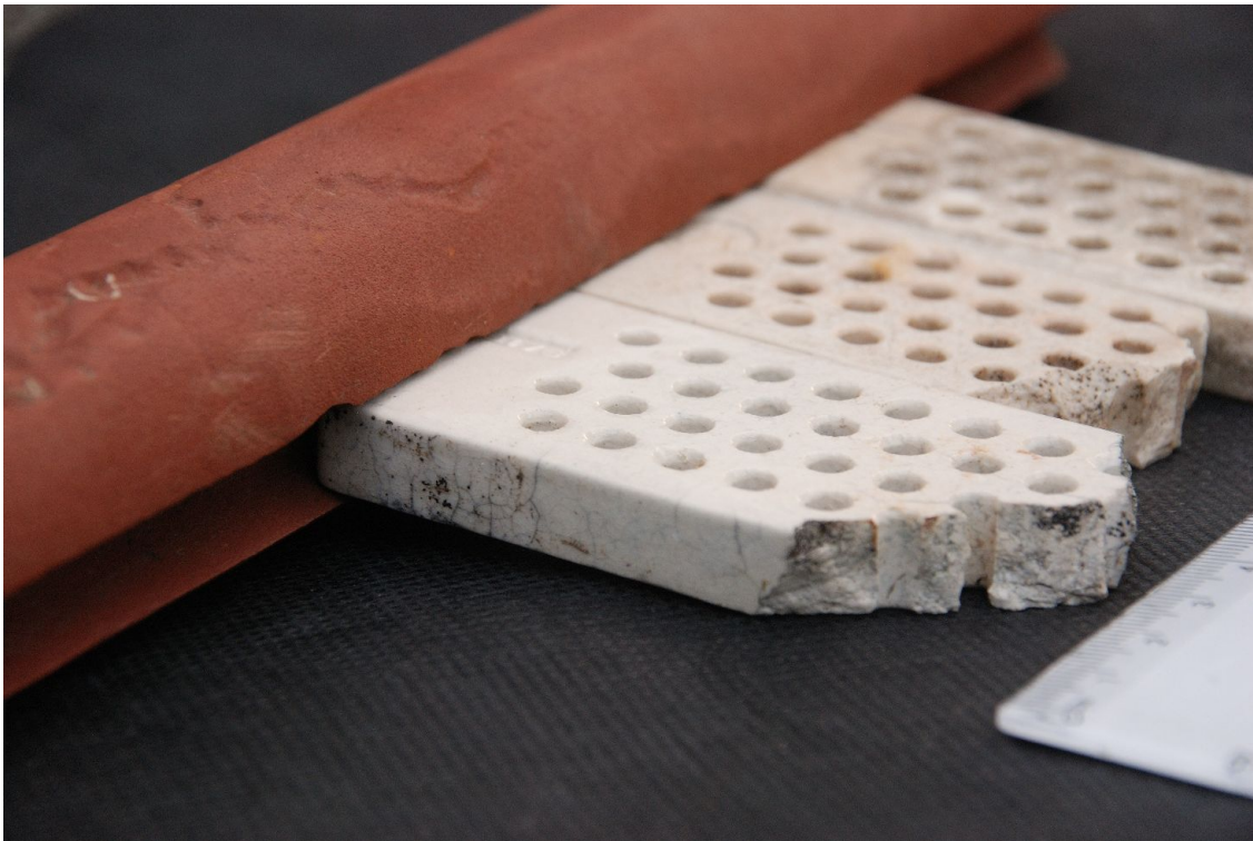
C8. Side view of the slotted spacer holder and how the insulators stacked together.
