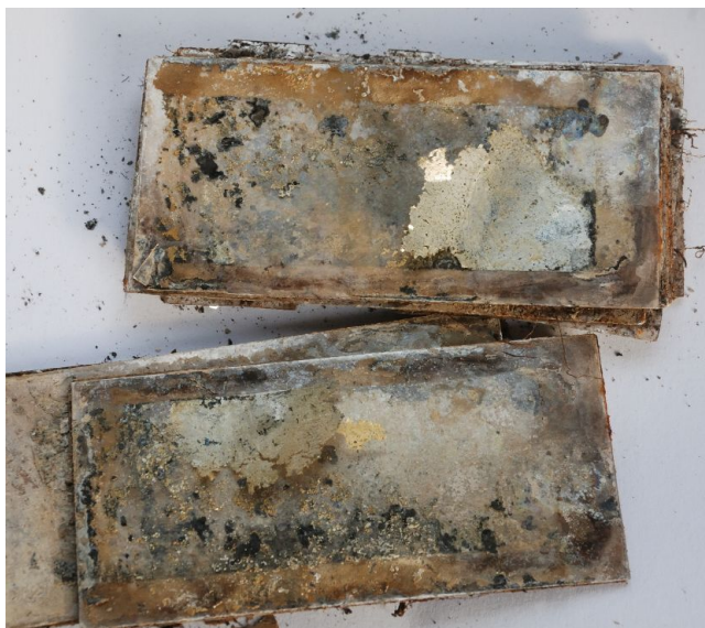
C30. Sheets of the capacitor, separated to reveal metal, probably silver foil plates, with detail at C31, below.
