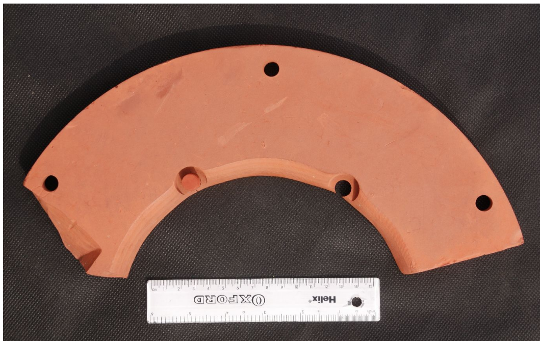
C12, below. Upper face. Width variable, 85-88mm; inner diameter = 7\frac{1}{4} " ; outer diameter = 14" ; thickness = 18mm. Scale = 15cm/6". Inner perimeter apparently hand-chamfered.
