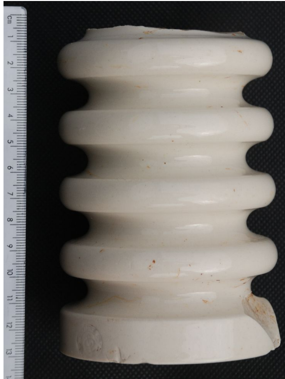
C23. Cylindrical ribbed insulator, bearing Taylor and Tunncliff impression (at lower left), found at the double inductor house. These had many uses, similar ones seen in use at C19 .
