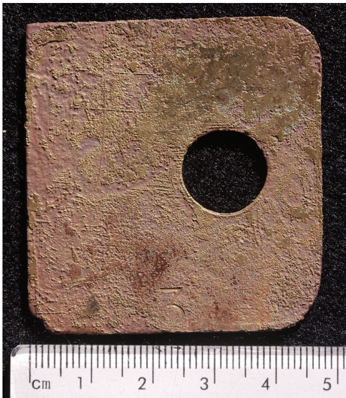
C22. Numbered connector tag, probably of an oil-and-glass capacitor from upper ATI house.
