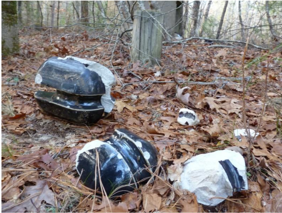
18. Egg insulator remains, identical to Carnarvon, except for the glaze colour, at Marion, MA, USA. Image by kind permission and © of Marian Howell via Sippican Lands Trust.
