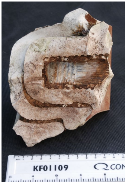
C26, a and b , below: some of the components still cemented together in a separate discovery. These probably formed part of the earth or feed line system.
