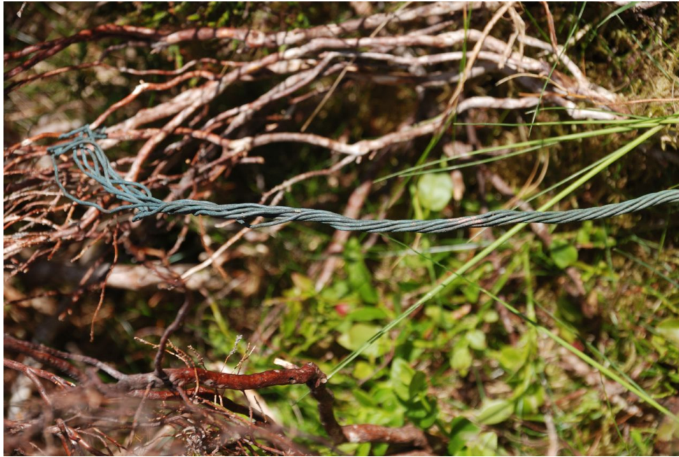
53. Remnant wire found at the upper end of the 1923 extension. This is 7, rather than the 6-stranded wire generally seen around the 1914 site, though 7 strand was originally specified for the 1914 antenna.
