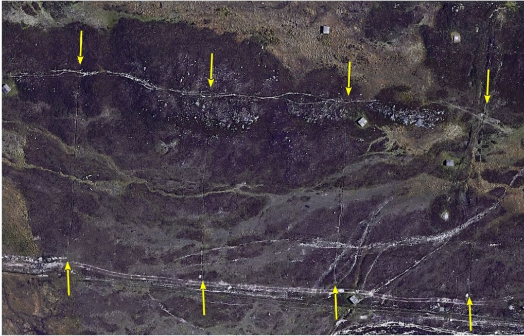
51. Arrows indicate obvious cuts in the ground running along a roughly N-S line between counterpoise masts (or existed beforehand). The cuts are also obvious from ground level.
