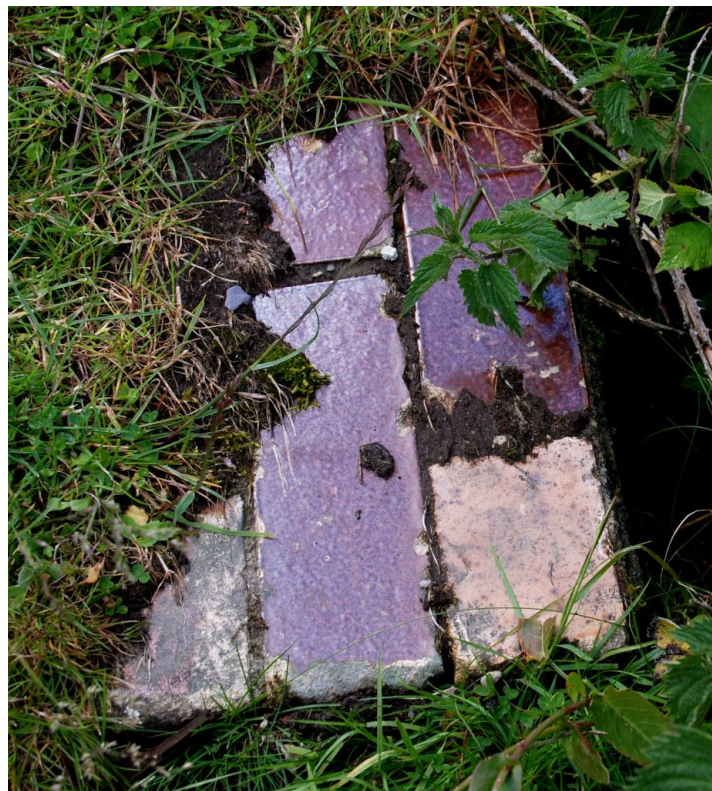
C34. Purple, vitreous-glazed wall tiles lying to the west of the transmitter building. These were once inside that building. An isolated such brick found nearby (C35, below, in orange glaze) bears impression of Leeds Fireclay Co Ltd (latter three characters obliterated, but known from example given at Grace's Guide to British Industrial History, accessed 17/08/2022). 'England' appears vertically between the deeper frog impressions. Leeds Fireclay Co was based in Wortley, Leeds, and active from 1889.
