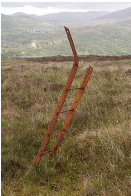
63. Part of a ladder that probably ran inside Mast 13 before it collapsed. A mast-connecting section running at 90 degrees to the plane of the rungs can be seen running, partly-buried to the left at ground level (and unseen, extending to the right also). It is thus thought to have been the topmost ladder section, emerging onto a platform, as all the other connections to the mast were in the same plane as the rungs.
