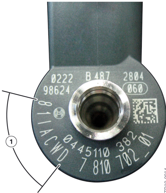
Injection quantity compensation EURO 5 solenoid injector .5
