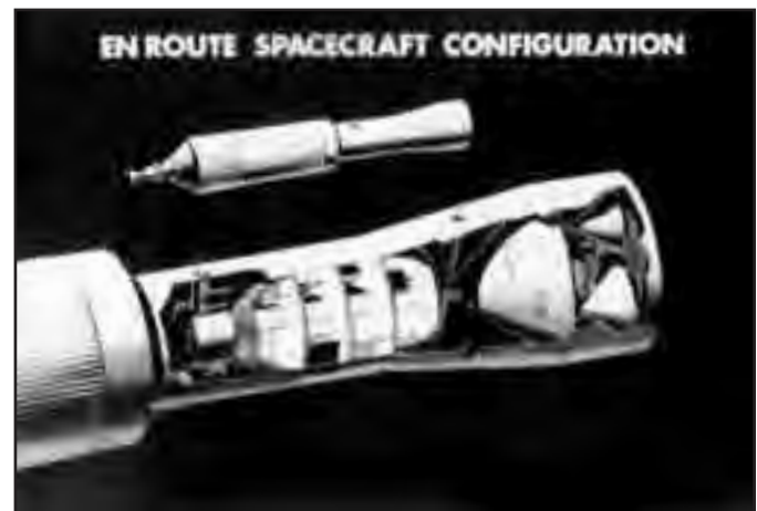
Figure 16—Compared with cramped Apollo spacecraft, the lodgings proposed for NASA's 1980s Mars ships were palatial. In this cutaway, note the four-deck Mission Module (center) and large conical Mars lander (right). (NASA Photo S-69-56295)
