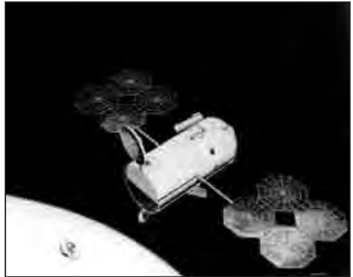
Figure 11—The 1967 Planetary Joint Action Group's Mars flyby spacecraft releases automated probes and deploys instruments. Close Mars flyby would last mere hours, but the astronauts would study themselves throughout the mission, helping to pave the way for future Mars landing expeditions. (NASA Photo S-67-5999)
