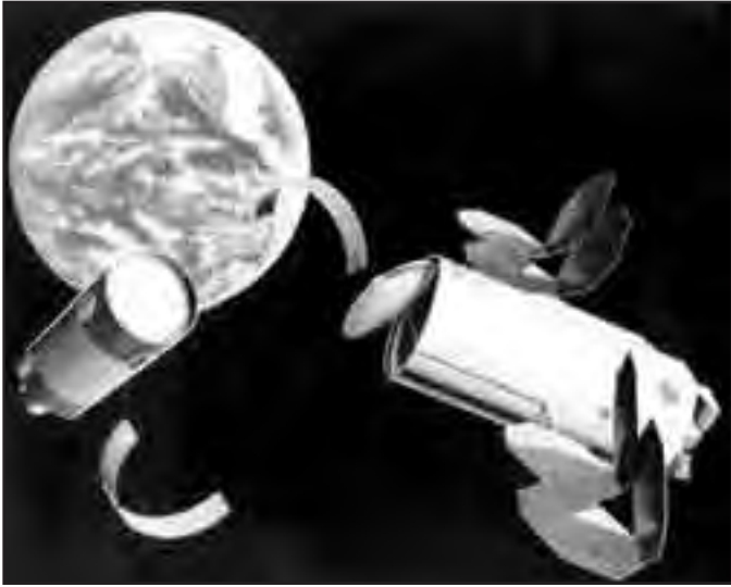
Figure 10—Following final S-IVB stage separation, the 1967 Planetary Joint Action Group's Mars flyby spacecraft deploys solar arrays and a dish-shaped radio antenna. (NASA Photo S-67-5991)
