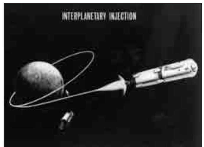
Figure 9—Three modified Apollo S-IVB stages burn one after the other to launch the 1967 Planetary Joint Action Group Mars flyby spacecraft out of Earth orbit. (NASA Photo S-67-5998)
