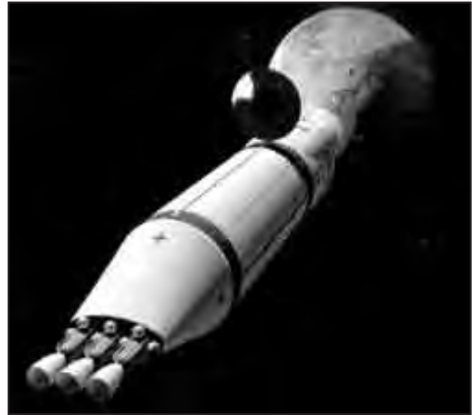
Figure 29—Nuclear stages in NASA's 1997 Mars plan included engines (left) based on revived 1960s NERVA technology. (NASA Photo S97-07843)
