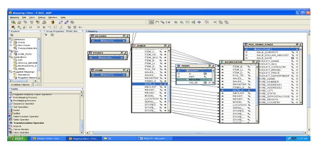
10] Connect the **DATE\_SOLD** attribute in the **OUTGRP1** group of the joiner to **D** attribute of the **INGRP1** of the trunk. Then connect the value attribute of the return output group from **TRUNC** operator to the **DATE\_SOLD** attribute if the INGRP1 group.
