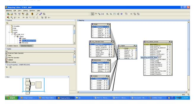
8] Click once on the header of the box to select it and the properties window. Click on the blank box to right of the **joint condition(...)** and write following query:
