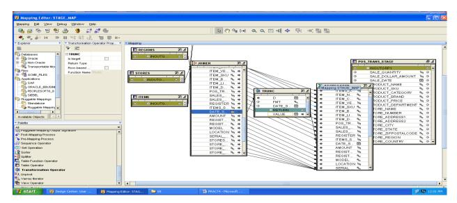
11] Select the aggregator operator and in the properties window we will click on the ellipse(...) on its right to open the **EXPRSSION BUILDER** FOR the **GROUP BY CLAUSE.** Write following query and click on the **OK** button.
