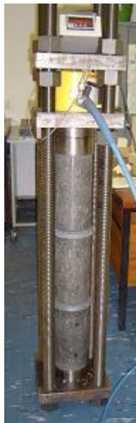
Figure 3.13 Creep Test Set-up
