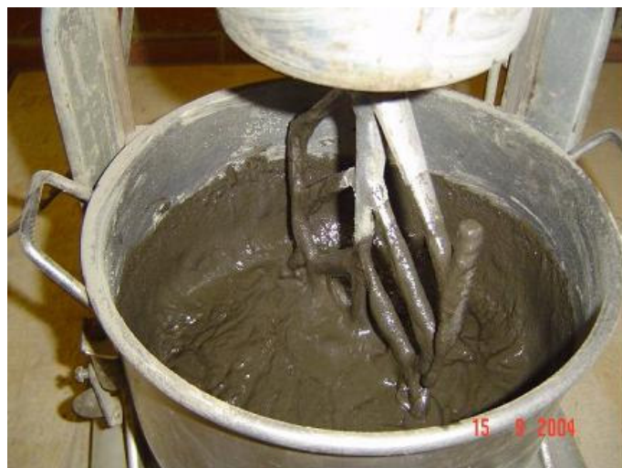
Figure 3.7 Fresh Geopolymer Mortar
