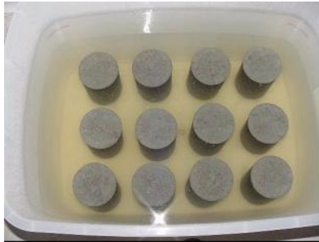
Figure 3.18 Specimens Soaked in Sodium Sulfate Solution
