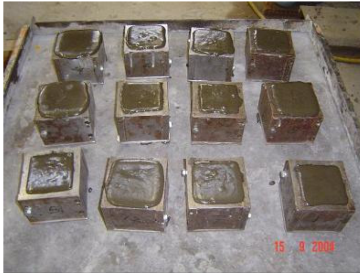
Figure 3.8 Compaction of Mortar Specimens
