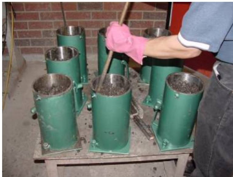
Figure 3.5 Compaction of Concrete Specimens
