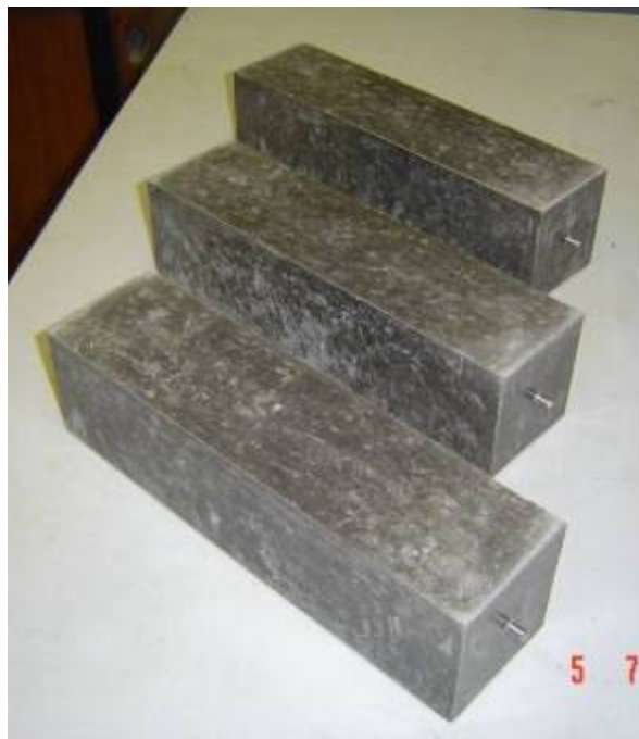
Figure 3.15 Specimens for Drying Shrinkage Test
