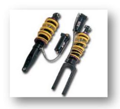
Bump means the upwards movement of the suspension, Rebound the downwards movement.
