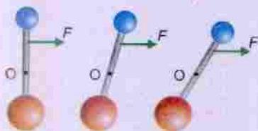
Figure 4.18: The system moves as well as rotates when a force is applied away from COM.
