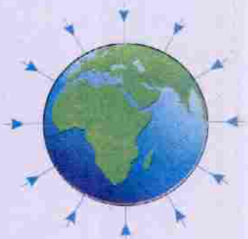
Figure 5.3: Gravitational field around the Earth is towards its centre.
