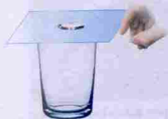
Figure 3.5: The coin falls into the glass as the card flicks away.
