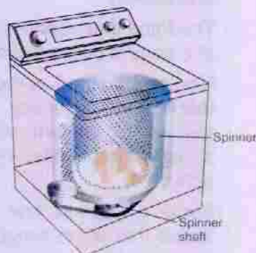
Figure 3.30: Dryer of washing machines has perforated wall.
