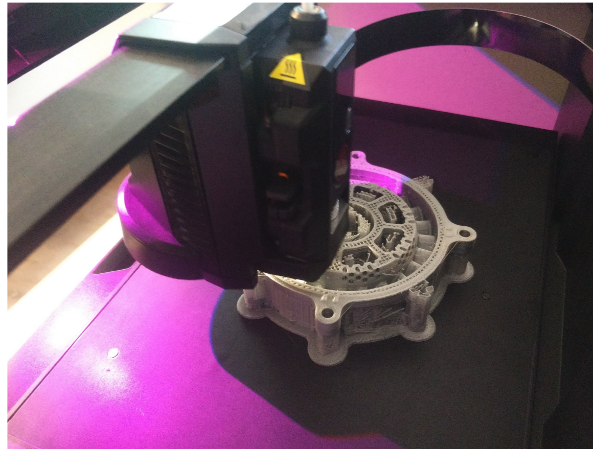
The school’s Makerbot Replicator+ printing out the motor mount. You can see the thick wall thickness and high infill.
