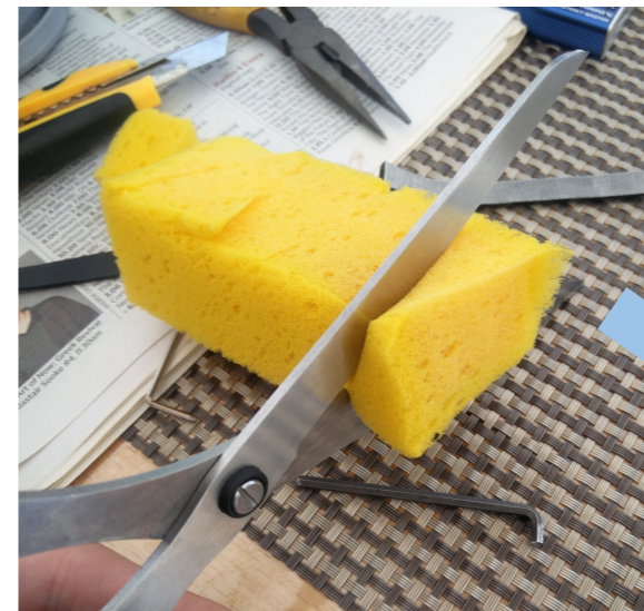
For my version of an acoustic liner to work, sponge has to be added into the inside of the mount so that the holes in the mount are met by sponge. The pieces were all cut from a regular consumer sponge which should do the job due to its open-pore characteristics.
