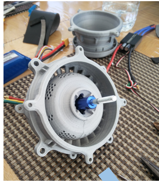
Testing if motor slides in and fits in correctly
