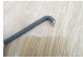
The hex key's short end was cut down so that it could fit inside the mount.
