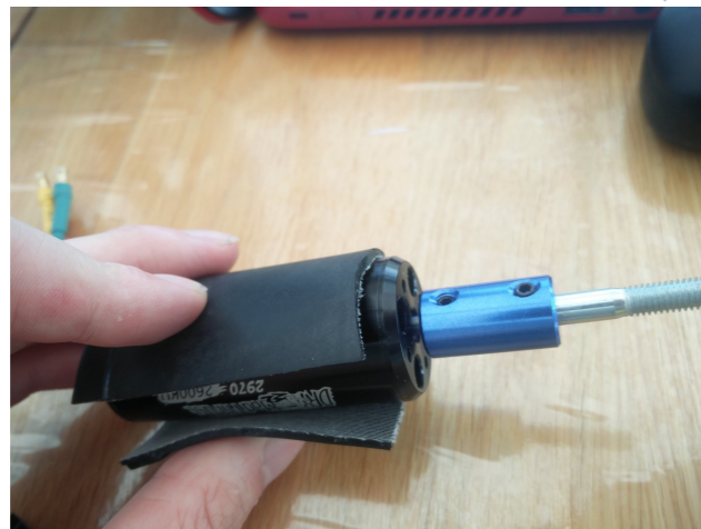
A strip of rubber was cut from a Wellington boot—the rubber likely to be neoprene. Silicone or even Sorbothane would've been preferred due to their greater vibration dampening properties but this neoprene piece was much more readily available at no extra cost and the rubber needing to be 2mm thick, the performance gains with the more expensive rubbers is likely to be minimal and hence not worth the delay and cost. The image shows me checking if the rubber piece is the correct size and will fit around the motor properly.
