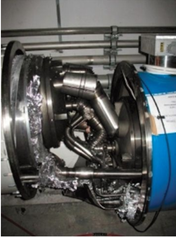
Damage to LHC magnets after the September 19 accident.
