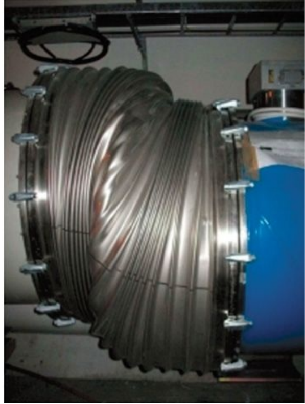
Damage to LHC magnets after the September 19 accident.
