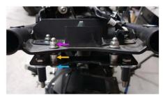
After fitting the body mount bracket, re-install the brake light using the two most rear bolts. Tighten all four bolts once brake light is fited
