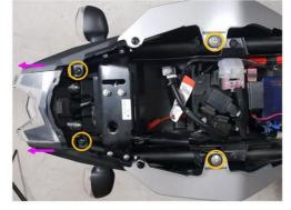
**STEP7**: Remove Latch Plate and Unplug Indicator Connectors
