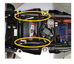
The extra cable length can be tucked along the sides of the storage tray and frame
