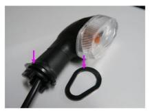
Fit supplied spacer to indicator
