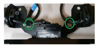
Feed indicator and licence plate light cables through rectangular holes on tail tidy
