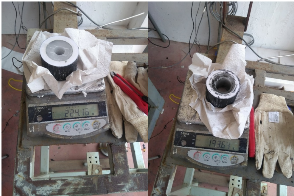
Figure 37 50 mm paraffin baseline grain before and after firing.
