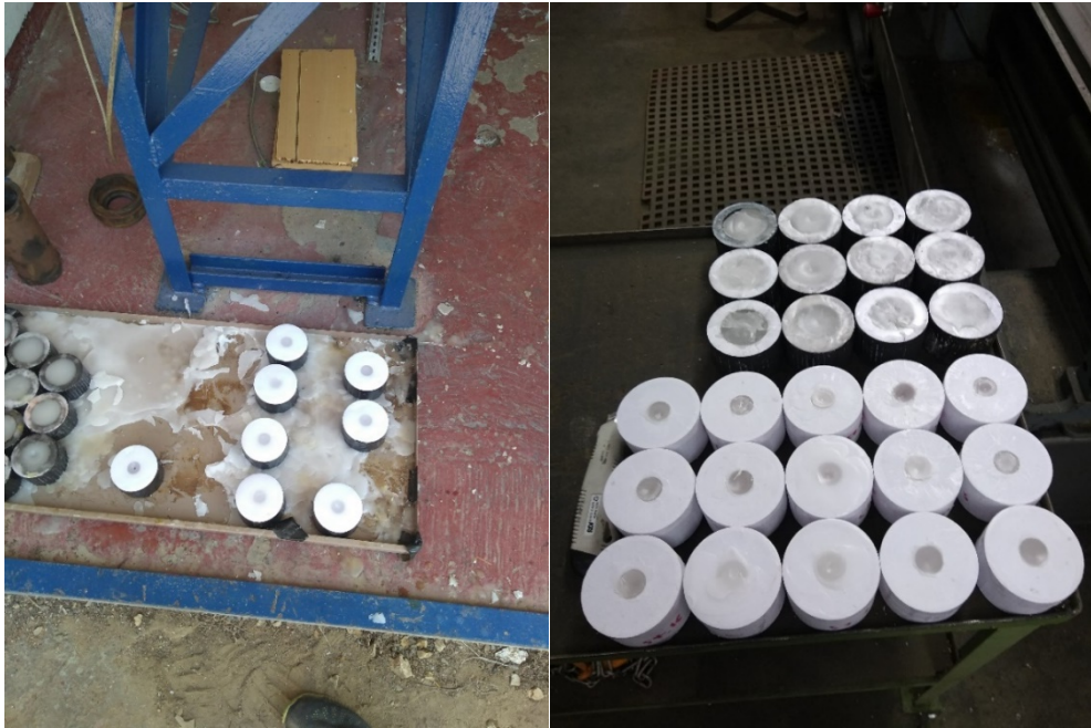
Figure 29 Grains on casting tray after filling (left) grains after being cleaned prior to machining (right).
