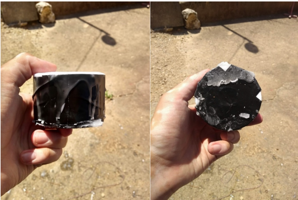
Figure 30 Skeleton filled with paraffin and displaying fabric tape utilization in casting.
