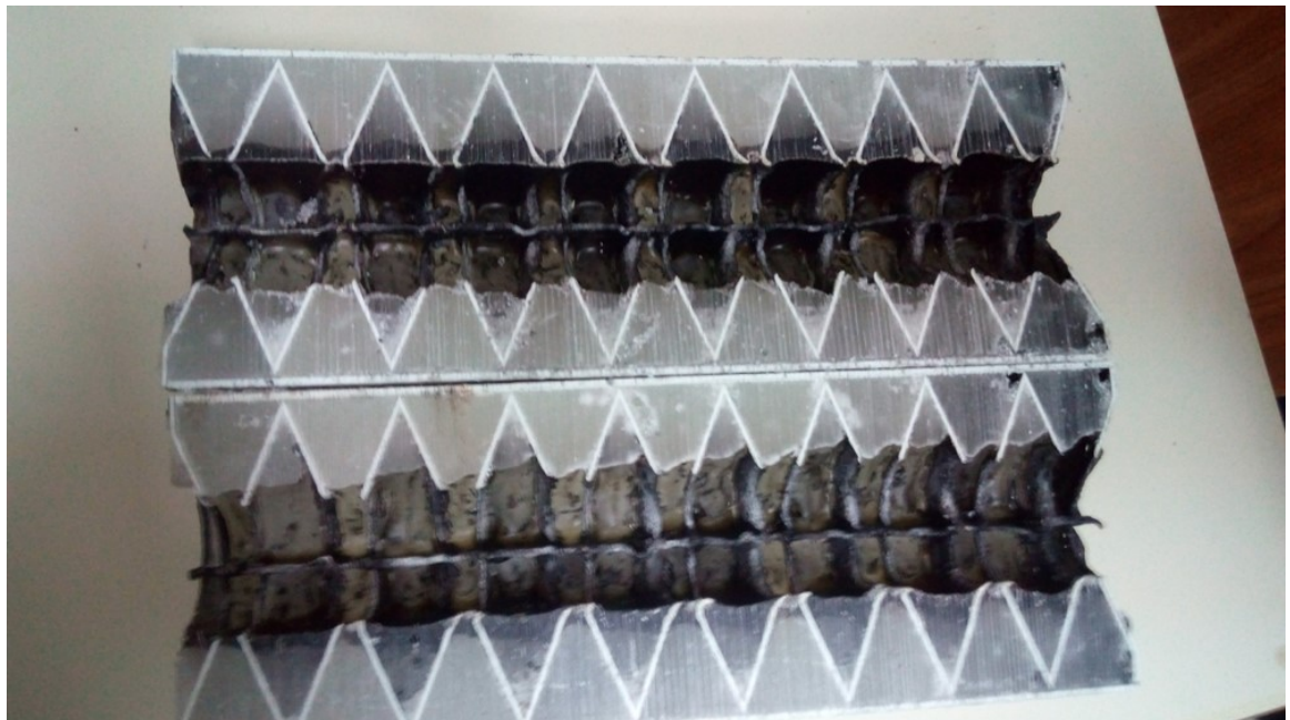
Figure 50 Cross sectioned Rafael Grain.
