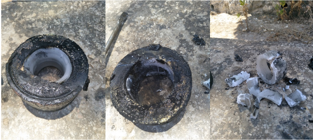
Figure 27 Pure paraffin grain before paraffin removal (left) cleaned of paraffin (center) paraffin removed from ABS (right).
