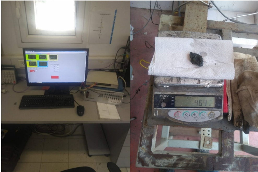
Figure 36 Data collection system, firing control box (left), and sample of unburned paraffin (right).
