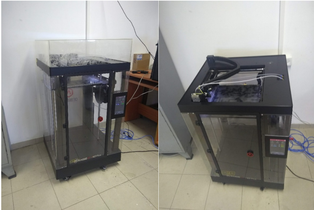
Figure 15 Raise 3d N2 Plus dual with Bondtech upgrade, without and with top enclosure.
