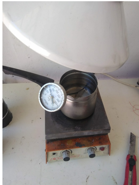
Figure 26 Molten paraffin with thermometer to achieve safe temperatures.
