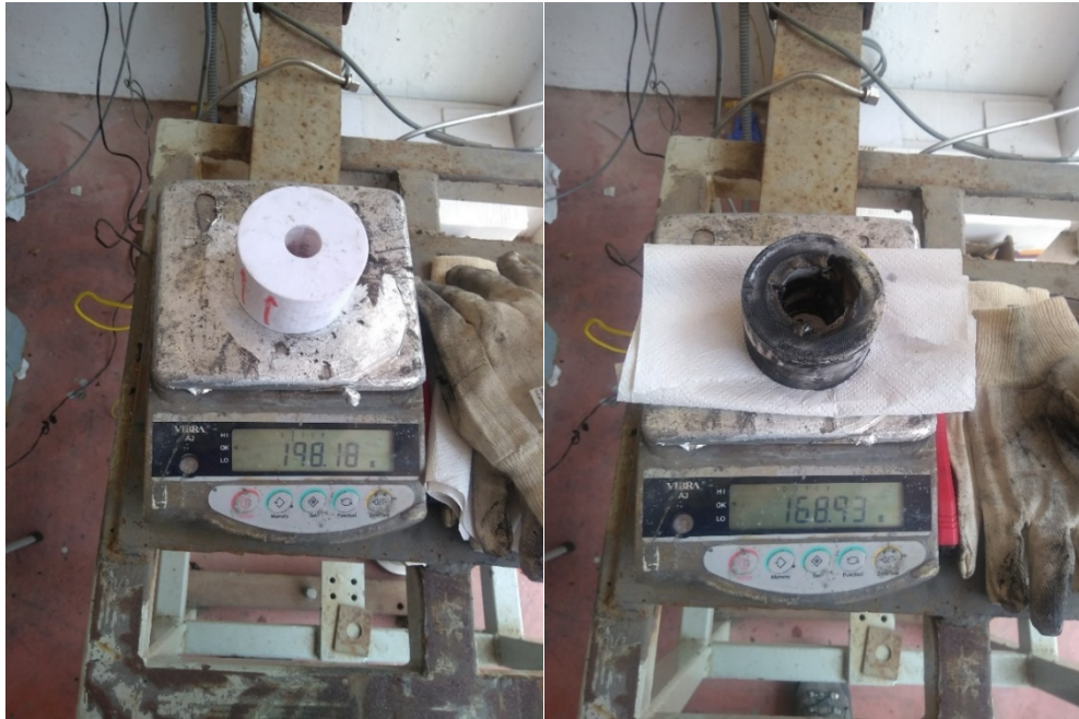
Figure 38 50 mm paraffin filled skeleton before and after firing.
