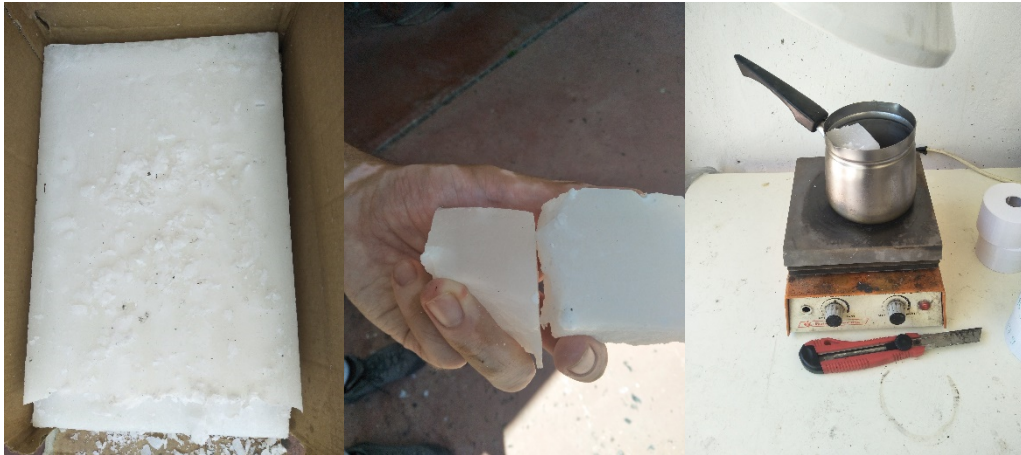
Figure 25 paraffin slabs (left), paraffin chunks (center), paraffin chunks in melting pot (right).
