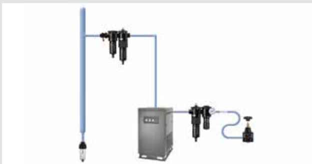
Figure 31. Shut-off valve, general purpose filter, oil removal filter, dryer, oil removal filter, regulator and precision regulator.
