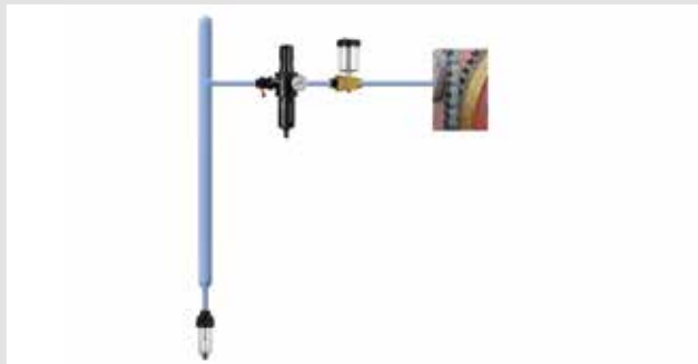
Figure 32. Shut-off valve, filter/reg + direct injection lubricator.
