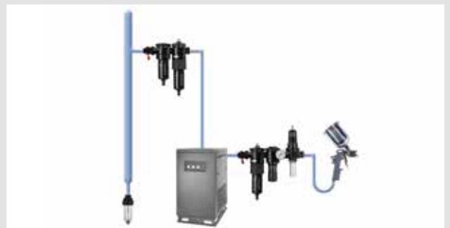
Figure 29. Shut-off valve, general purpose filter, oil removal filter, dryer, oil removal filter, regulator, relief valve.
