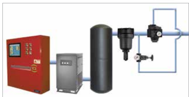
Typical compressor installation
