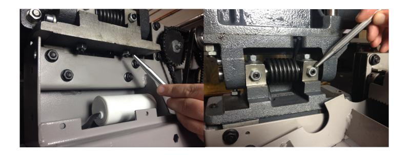
Adjust the castle nuts in relation to the hinge adjustments so that the cast-iron tables are even across the cutter block.
