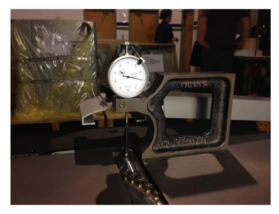
Measure the cast-iron to the cutterblock on the hinge-side first and the front side second.
