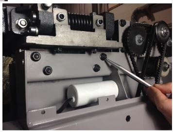
Loosen the four bolts and use the two worm screws to adjust the height of tables.
