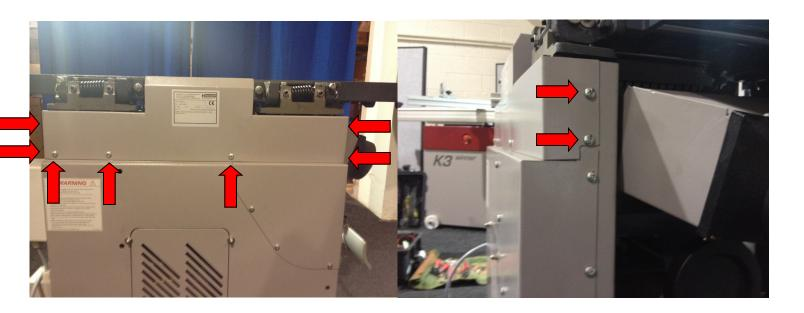
To access the adjustment bolts on the hinges, remove the back panel comprising of nine screws. (Two screws are not shown as they are located on the opposing side)
