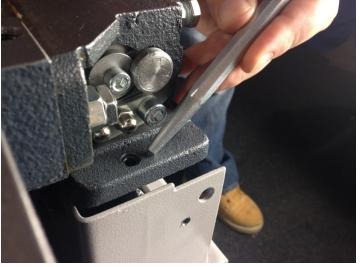
Use the four set screws on the hinge-pin to make fine adjustments and to make the infeed and outfeed tables parallel to the cutterblock.
