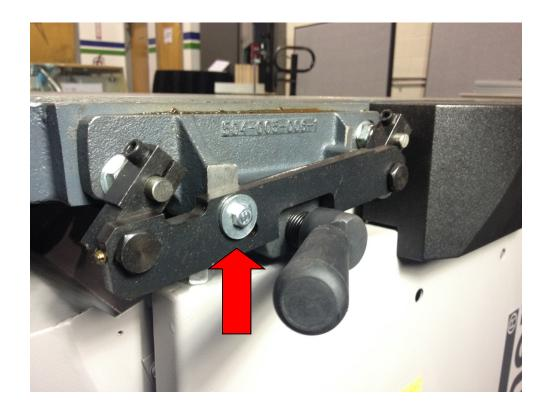
Loosen bolt (indicated above) to adjust the outfeed table up and down. Adjust table, using wrench, until bolt is set within the middle of its guide.
