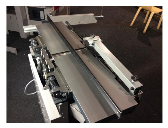
Once the outfeed table is level and parallel to the cutter block, use a straightedge to level the infeed table.
