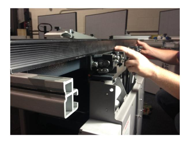
Place the straightedge on the cutter block assembly and confirm that the tables are coplanar with the cutter block assembly.
