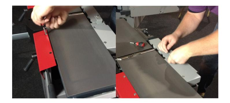
There are four panels that can be removed from the top side: two covering the hinges, and two covering the kip levers.
