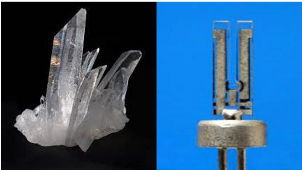
Figure 1.6 at the left is the natural Quartz crystal and at the right is the quartz tuning fork (Google).
