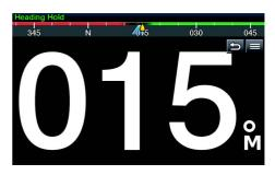
Heading Hold mode is a feature to navigate with the bow direction fixed.
