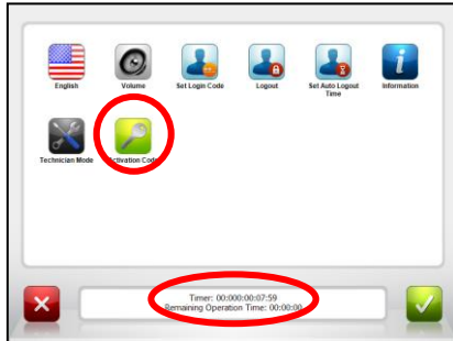
Figure 5-47: Tools Screen - Activation Period is ON (date limited)
