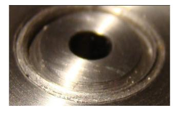
The images above illustrate the different finishes provided by traditional anvil staking tools and Tri-roller swaging tools. The roll stake tri-roller tool (Fig 1) has provided an even, smooth and mirror-like surface to the swaging lip on the bearing. Virtually no gap
