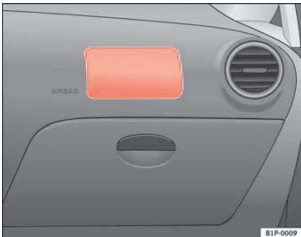
Fig. 18 Front passenger airbag located in dash panel
