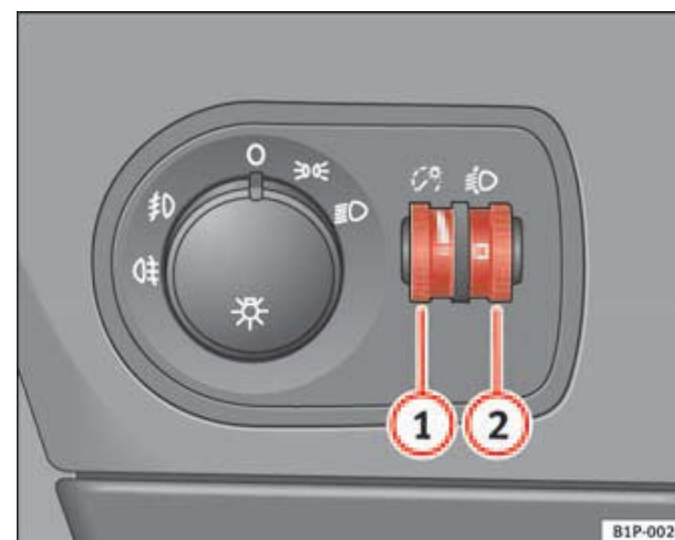
Fig. 74 Detail of the dash panel: Regulation for instrument and switch illumination and headlight range control ▶
