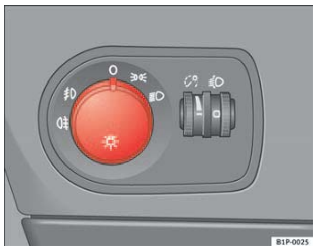
Fig. 72 Detail of the dash panel: Switch for lights, fog lights and rear fog light
