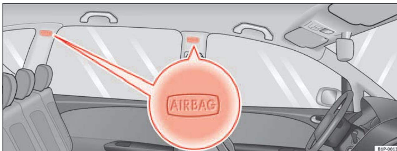
Fig. 23 Location of left curtain airbag
