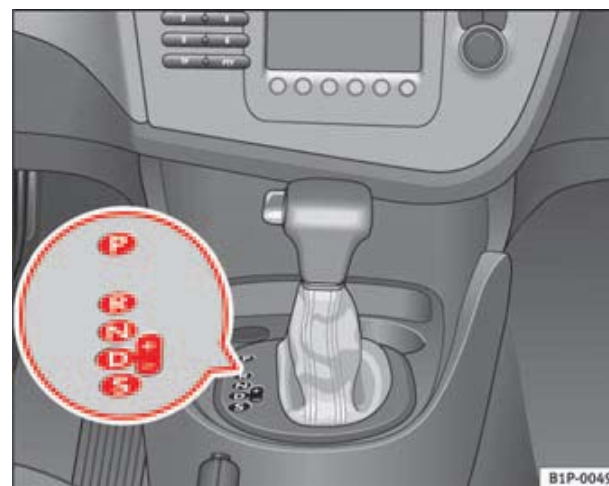
Fig. 118 Section of centre console: selector lever on cars with an automatic gearbox / direct shift gearbox
