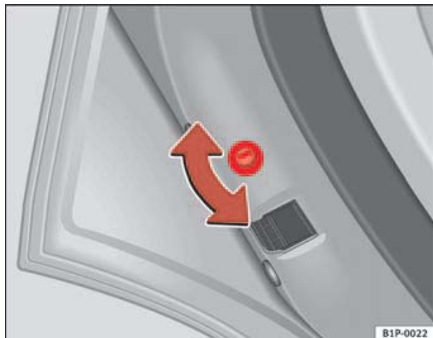
Fig. 60 Child safety lock on the left-hand side door
