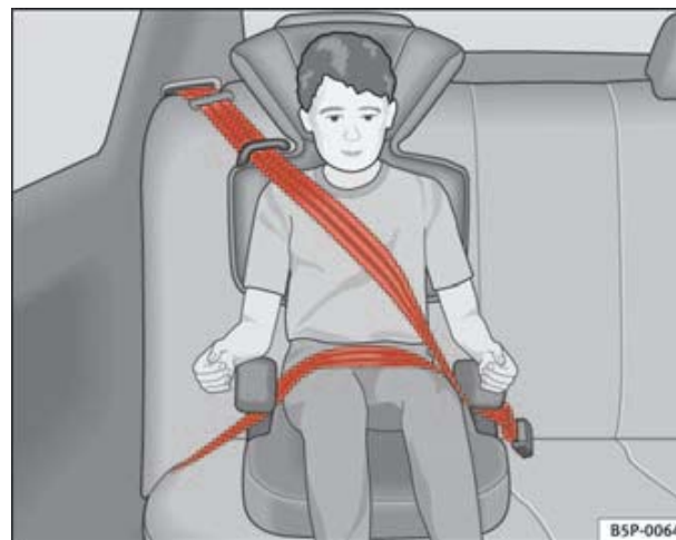
Fig. 29 Forward-facing child seat installed on rear seat.
