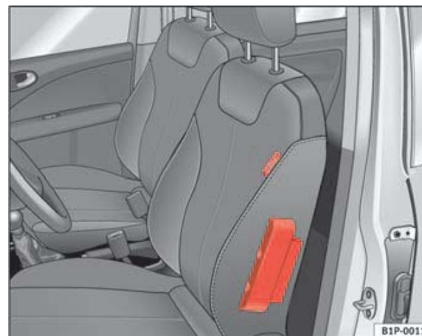
Fig. 21 Side airbag in driver seat
