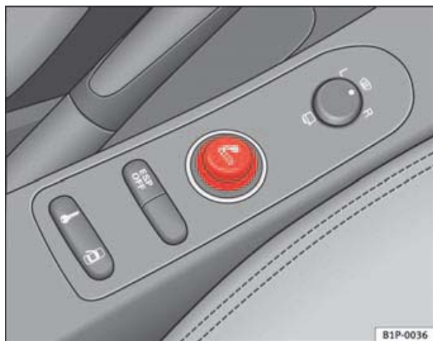
Fig. 99 The cigarette lighter is located in the electric socket on the front of the centre console
