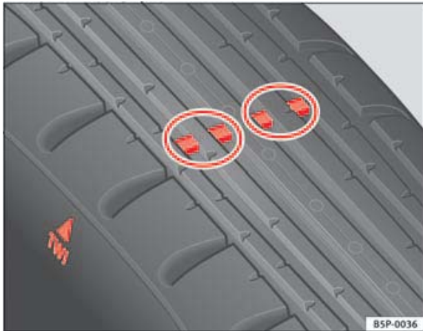
Fig. 151 Tyre tread wear indicators
