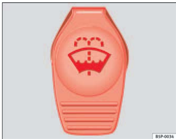
Fig. 147 In the engine compartment: Cap of windscreen washer fluid reservoir.
