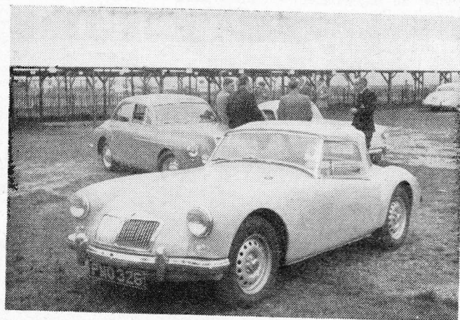
DIFFERENT APPROACHES to the design of a sporting two-seater were exemplified in the G.T. Allard (left) and the Twin-Cam M.G.A. (right). The Allard is a big car (in fact there are two occasional seats in the back) and is a luxurious machine, powered by the 3½-litre Jaguar engine. The new M.G. is strictly a sports car and is propelled by the noisy, but extremely potent, 2 o.h.c., 1,600 c.c. B.M.C. engine; the performance of the two cars would be fairly comparable.
