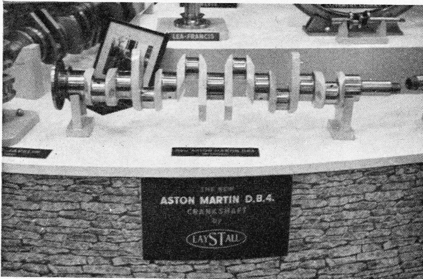
CRANKSHAFT for the potent new DB4 Aston Martin had a place of honour on the Laystall stand.
