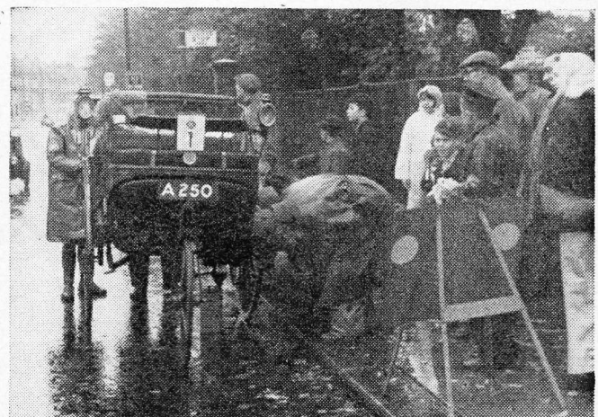
THE OLDEST CAR IN THE RUN. The 1888 Benz of Dr. T. Morrison-Scote and C. F. Caunter halts for hand greasing. This car runs on iron "tyres" and was allowed to start half an hour early.
