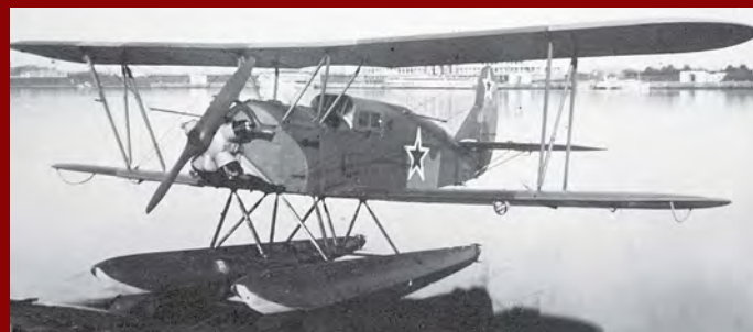
ABOVE: The float-equipped Po-2LP at Aviation Repair Base No 402 at Bykovo in the Moscow area.
