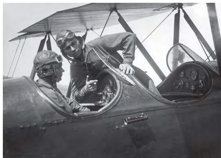
ABOVE: An instructor explains the purpose of the few instruments in the aft cockpit to his trainee. The forward cabin features a non-standard instrument panel accommodating a starting magneto.
