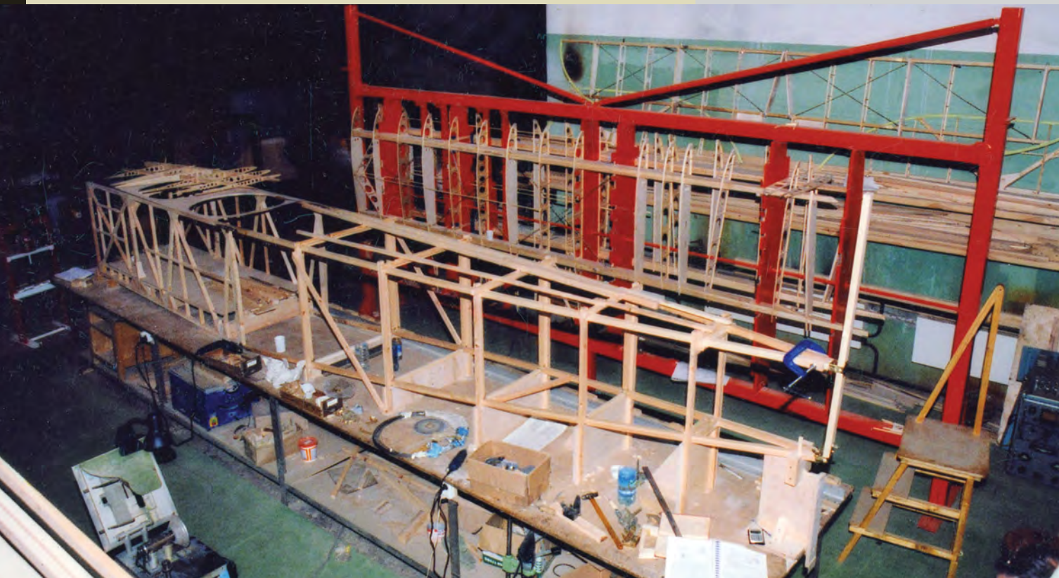
ABOVE: Assembly of a Po-2 fuselage frame during a recent restoration in Russia. In the background is a rig for the wing assembly.
