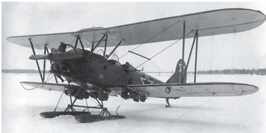
ABOVE: U-2VS c/n 4504 with an M-11D engine, manufactured at Factory No 387 in October 1943. The photo was taken during state testing, which took place from 21 November 1943 to 13 January 1944.
