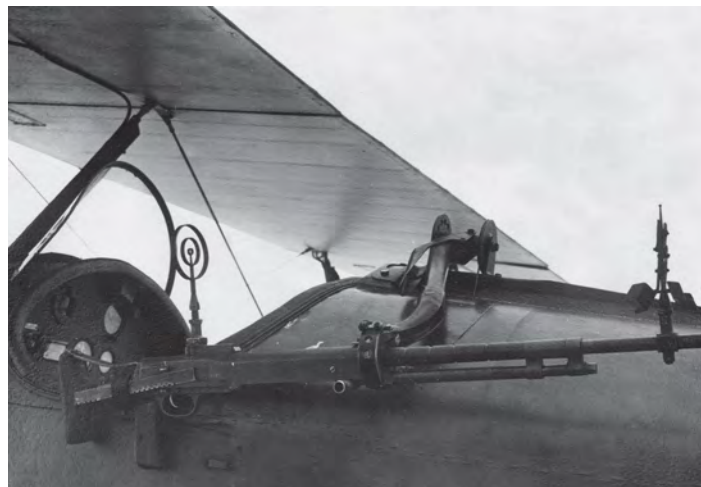
ABOVE: An MAKF-4 muffler/flash reducer on an artillery observation U-2 in autumn 1943. LEFT: A DT machine gun (without its cartridge tray) in the stowed position on the pintle mount of U-2VS c/n 4504.
