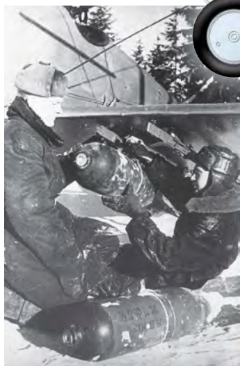
ABOVE: The attachment of 50kg (110lb) bombs to a U-2's underwing racks.
