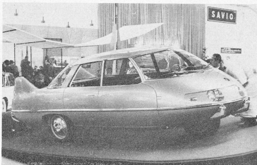
CAR of the future (1): This is the Pininfarina "X", which boasts a single front wheel (for steering), a single rear-wheel (for driving) and two at the sides (for balancing).
