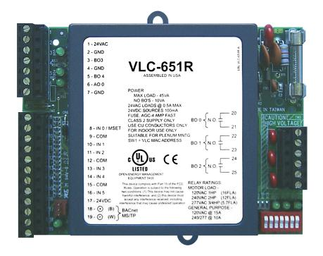
The Alerton BACtalk® VLC–651R is a versatile, fully programmable BACnet-compliant field controller. With three software-controlled high-current relays, the VLC-651R is well suited for unit ventilator and fan-coil applications, or any application that requires multi-speed fan or motor control. As a native BACnet controller, it integrates seamlessly with your BACnet system, communicating on a BACnet MS/TP LAN at up to 76.8 Kbps.
