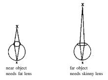
The squeezing is controlled by the focusing reflex, a feedback loop that adjusts the shape of the lens until the fine detail on the retina is at a maximum. (The circuit is similar to the one used in some autofocus cameras.) Poorly focused movies are annoying to watch because the brain keeps trying to eliminate the blur by accommodating the lens, a futile gesture.
