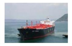
Chemical tanker - Specially designed for the transport of chemicals.
