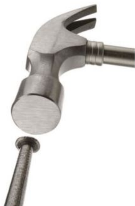
FIGURE 10.3.1 A hammer hitting a nail is a good example of an action–reaction pair and Newton's third law.
