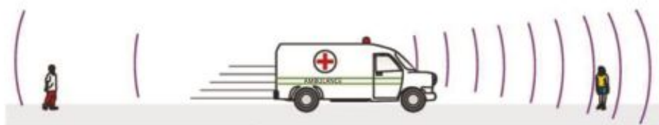
FIGURE 5.1.8 The Doppler effect. A moving source of sound produces a shorter wavelength and higher frequency sound in front, but a longer wavelength and lower frequency one behind.
