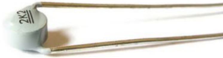
FIGURE 4.2.5 The resistance of a thermistor changes with its temperature.
