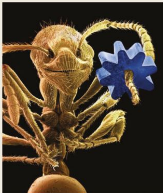
FIGURE 7.3.8 Gears like this one can be produced by using deep-etch lithographic techniques. They are used to build micromachines.
