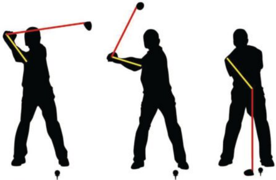
FIGURE 18.3.13 The double pendulum model of a simple golf swing showing upper (yellow) and lower (red) pendulums.
