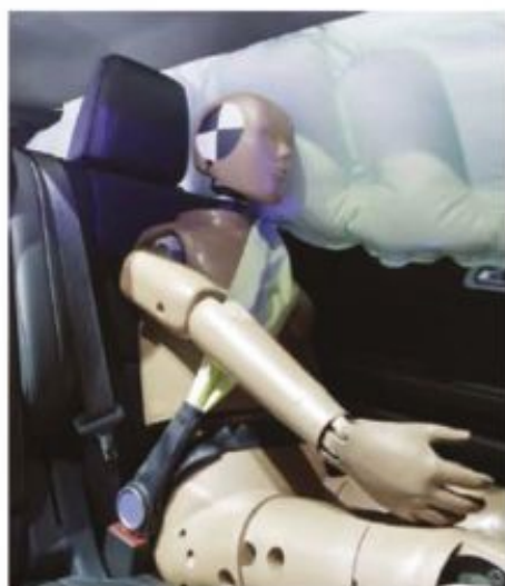
FIGURE 14.1.1 Researchers use crash test dummies to simulate the effects of high-speed car crashes in order to understand the impacts on the human body.
