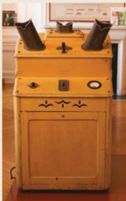
FIGURE 16.1.8 In the first half of the twentieth century, some shoe shops had X-ray machines that were used to see if a shoe was a good fit. These machines would have produced soft X-rays.
