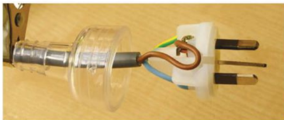
FIGURE 4.3.2 This three-pin plug shows the correct colour code used: brown for active, blue for neutral and green/yellow for earth.
