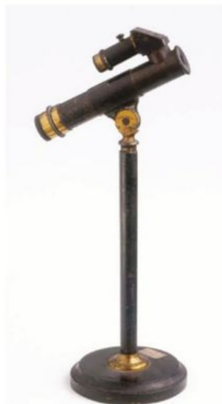
FIGURE 13.1.4 A model of the spectroscope invented by William Crooke in the nineteenth century.
