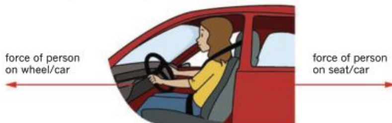
FIGURE 10.1.5 This driver is applying internal forces on a car. These internal forces will balance and cancel each other.
