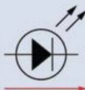
FIGURE 4.2.15 An LED circuit symbol. Current will flow through the LED in the direction given by the red arrow.
