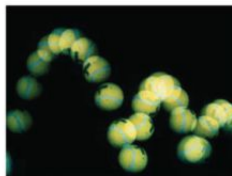
FIGURE 18.1.3 After each bounce, the ball has less energy. The ball has less speed after a bounce and also bounces to a lower height. The COR is less than 1.
