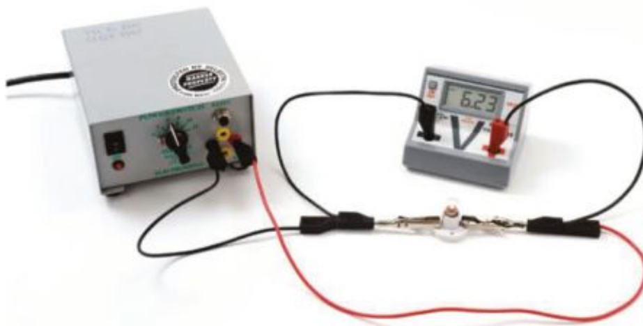
FIGURE 3.3.8 A voltmeter measures the voltage change (in this case, 6.23 V) across a light globe.
