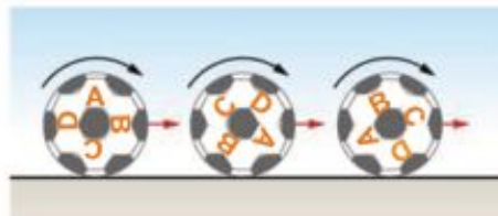
FIGURE 18.2.3 For a rolling ball, the surface of the ball and the ground are stationary relative to each other while they are in contact.
