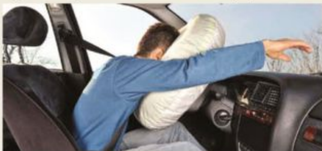
FIGURE 10.6.3 Airbags can prevent injuries by extending the period of time you take to stop.
