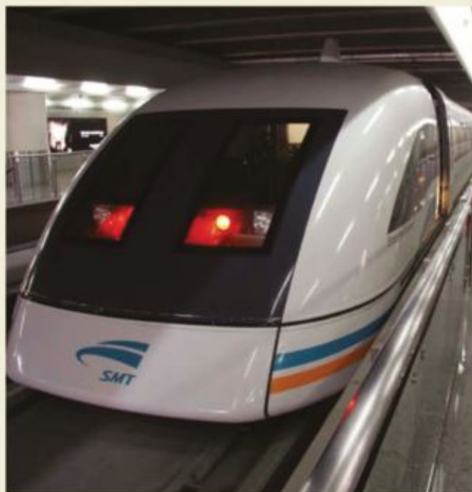
FIGURE 10.1.8 This magnetic levitation train in China rides 1 cm above the track, so the frictional forces are negligible. The train is propelled by a magnetic force to a cruising speed of about 430 \text{ km h}^{-1} .
