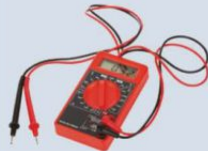
FIGURE 3.3.9 A digital multimeter can be used as either an ammeter or a voltmeter.
