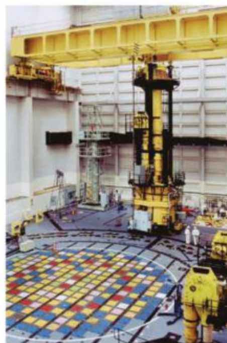
FIGURE 15.1.6 Inside a nuclear power station. The coloured squares provide access to the core that contains rods of uranium. Control rods are inserted into the reactor via the heat generated by the core. Control rods are inserted into the reactor via the coloured squares to control the amount of heat generated.
