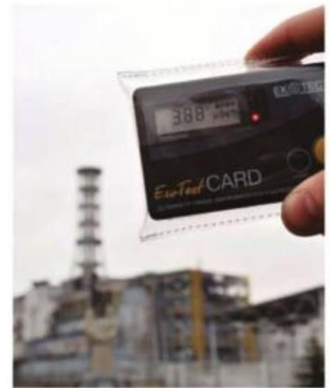
FIGURE 16.2.1 A dosimeter used to monitor gamma radiation exposure.
