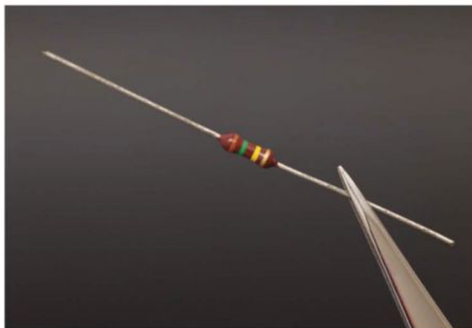
FIGURE 3.4.7 Common resistors are electrical devices with a known resistance. The coloured bands indicate the resistor's resistance and tolerance.
