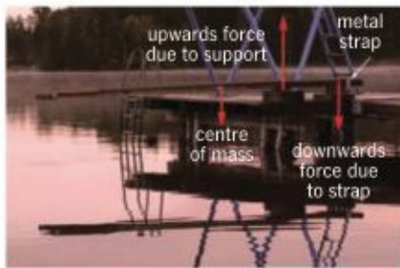
FIGURE 11.3.7 A diving board showing that a metal strap is needed to provide the downwards force on the fixed end of the board.
