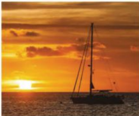
FIGURE 11.3.4 To keep this mast in rotational equilibrium in relation to its base, stainless steel cables (stays) attached to it must provide opposing torques on the mast.
