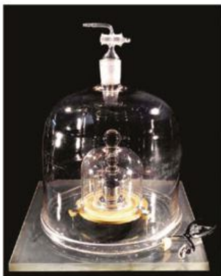
FIGURE 8.5.1 All mass in the world is compared to this small piece of platinum–iridium alloy held in a sealed vault in Paris.
