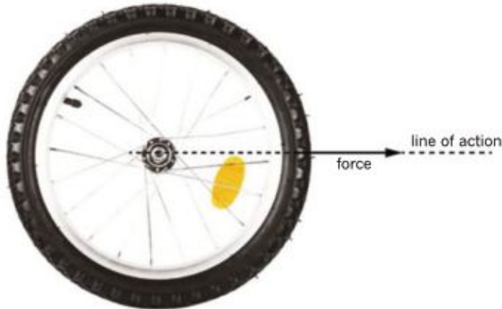
FIGURE 11.1.4 When the line of action of the force passes through the pivot point, the wheel will not turn.
