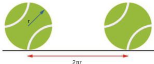
FIGURE 18.2.9 The roll distance is equal to the circumference for a full revolution of a ball.
