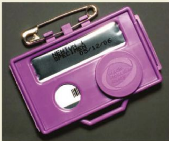
FIGURE 6.2.10 Thermoluminescent dosimeters are used by doctors, radiologists and scientists who work with radiation to monitor their exposure levels.
