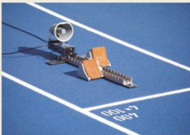
FIGURE 9.1.4 Starting blocks are fitted with pressure sensors to detect false starts.
