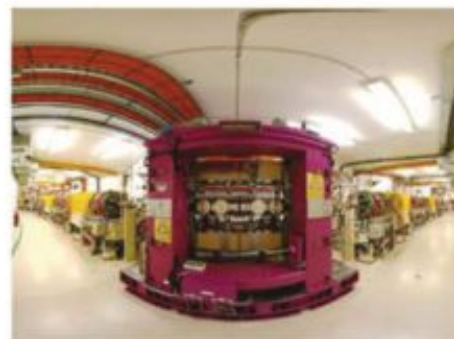
FIGURE 17.1.5 The booster to storage ring transfer line in the Australian Synchrotron.
