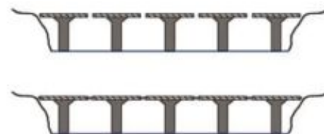
FIGURE 11.3.6 Each beam in the cantilever bridge is fully supported by the pillar below the beam. By connecting the beams no added support is provided.
