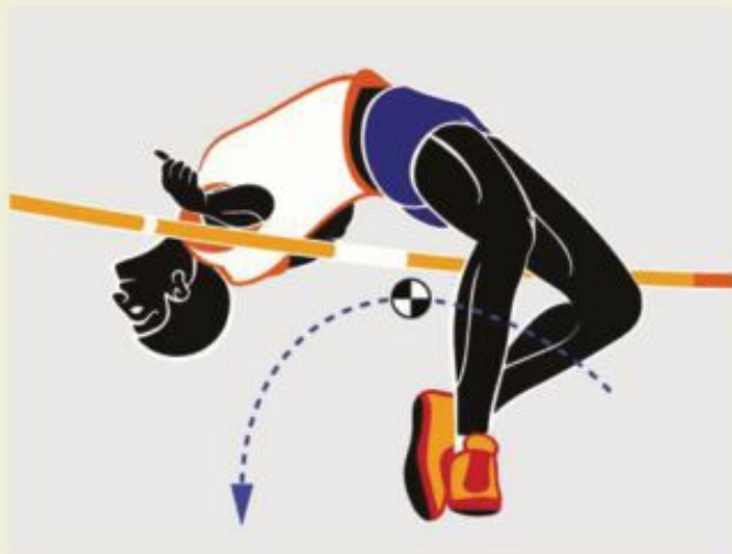
FIGURE 12.2.6 The path of the centre of mass of the high jumper (shown by the dashed curve) passes below the high jump bar.
