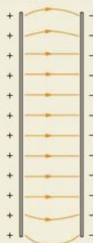
FIGURE 3.3.6 Electric fields can be represented by lines showing the direction of the field. The closeness of the lines suggests the strength of the field.
