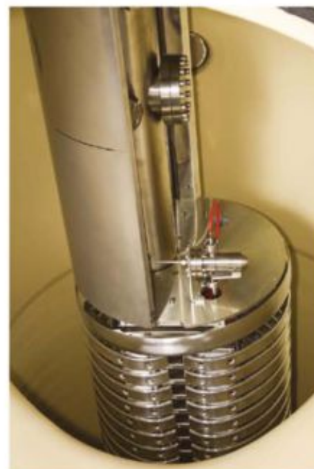
FIGURE 17.3.2 The interior view of an opened ion accelerator.
