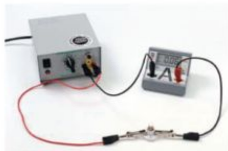
FIGURE 3.2.7 A digital ammeter (labelled with an A) measures current in a circuit.
