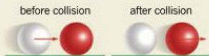
FIGURE 18.1.8 Since collisions between billiard balls are nearly elastic, both momentum and kinetic energy are transferred from the moving ball to the stationary ball.
