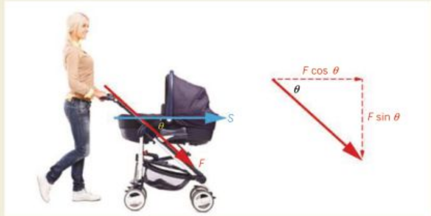
FIGURE 12.1.6 The force applied by the person pushing the pram can be resolved into a horizontal force and a vertical force.
