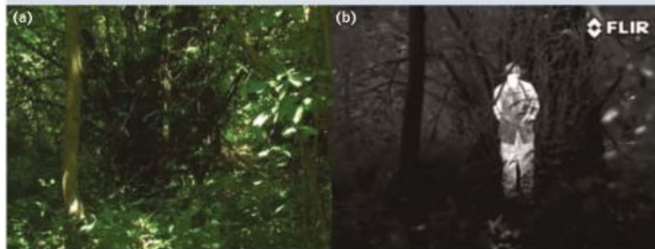
FIGURE 1.6.4 This person is difficult to see normally (a), but they are warmer than the trees surrounding them and produce a stronger infrared emission, which the thermal imaging device is able to detect (b).
