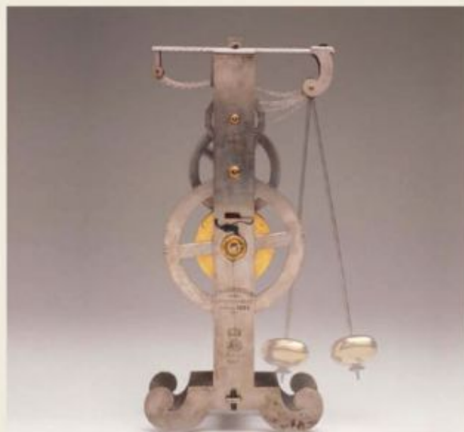
FIGURE 18.3.8 A model of a pendulum clock designed by Galileo.
