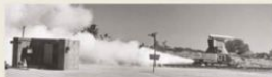
FIGURE 9.2.3 The rocket-powered sled used to test the effects of acceleration on humans.
