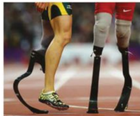
FIGURE 14.5.3 Single and double amputees wearing carbon fibre laminate running blades.
