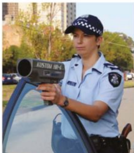
FIGURE 19.2.2 To avoid a systematic error, make sure that you are using measuring equipment correctly. Laser speed guns, for example, need to be placed on a stationary support so the aim point is held on a single target point for the duration of the read.
