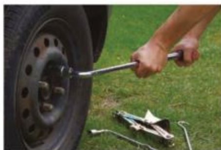
FIGURE 11.1.10 Removing a tyre with an extended handle spanner will increase the torque on the nut.
