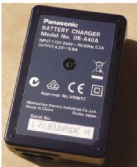
FIGURE 4.3.8 The double square symbol indicates that this appliance has double insulation and does not use an earth connection.
