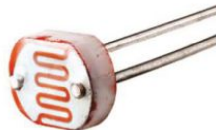
FIGURE 4.2.8 The resistance of a light-dependent resistor changes depending on how much light is falling on it.
