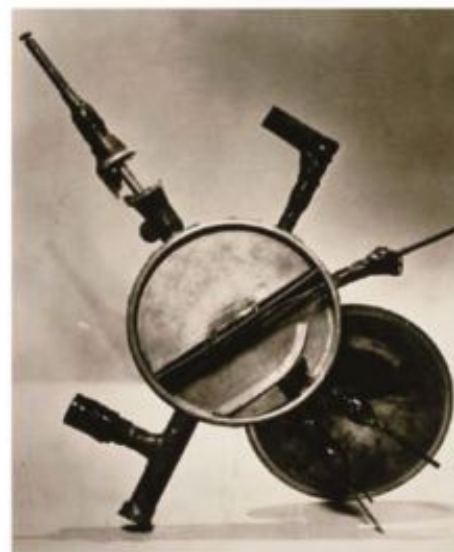
FIGURE 17.2.2 In 1930, physicist Ernest Lawrence built the first successful cyclotron, at Berkeley, California. It was just 13 cm in diameter and it accelerated protons to an energy of 80 keV.
