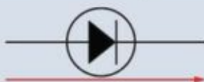
FIGURE 4.2.14 The red arrow under the diode symbol shows the direction of current flow.
