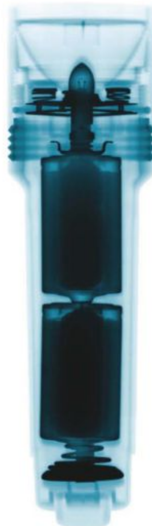
FIGURE 3.3.4 An X-ray image of the internal structure of a torch. The bulb and two batteries are clearly visible.
