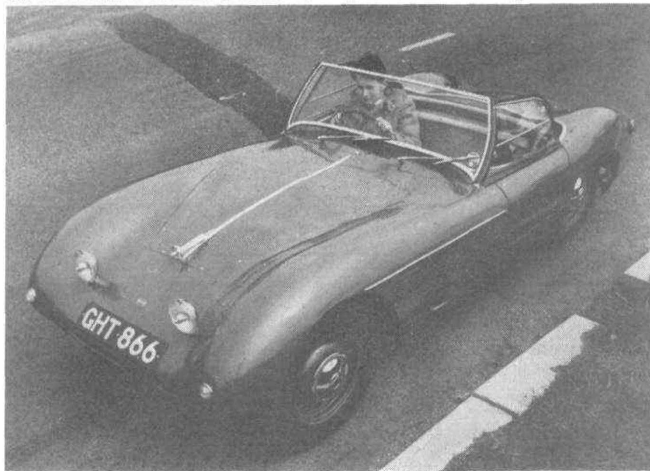
THE last production Buckler was the DD2 which would accept a wide range of proprietary fibreglass bodies. The above example has a Microplas Mistral shell.
