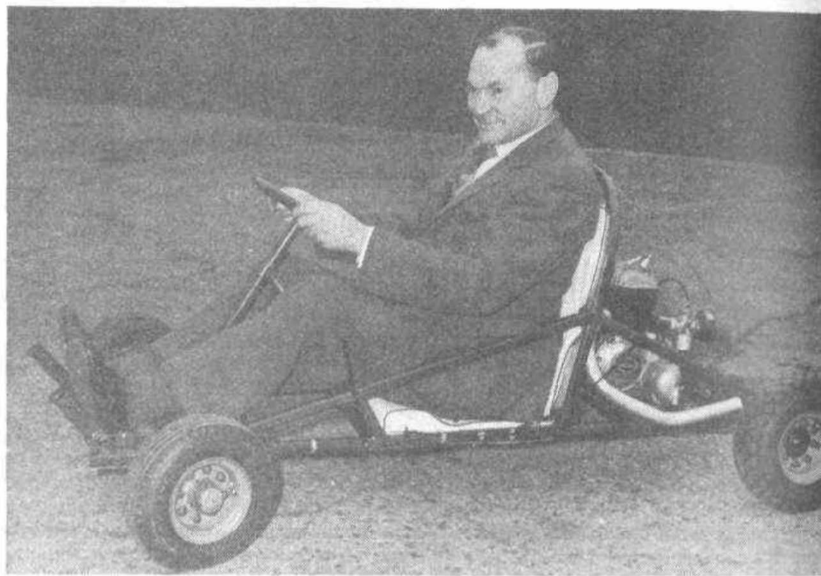
KARTING was a natural outlet for Buckler's philosophy and (above) Derek is seated in his Villiers-engined prototype circa 1960. Production models were low, sleek and handsome.
