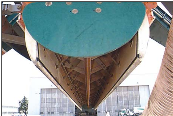
Figure 4 Drop-doors on the firebombing tank in the fully-open position
