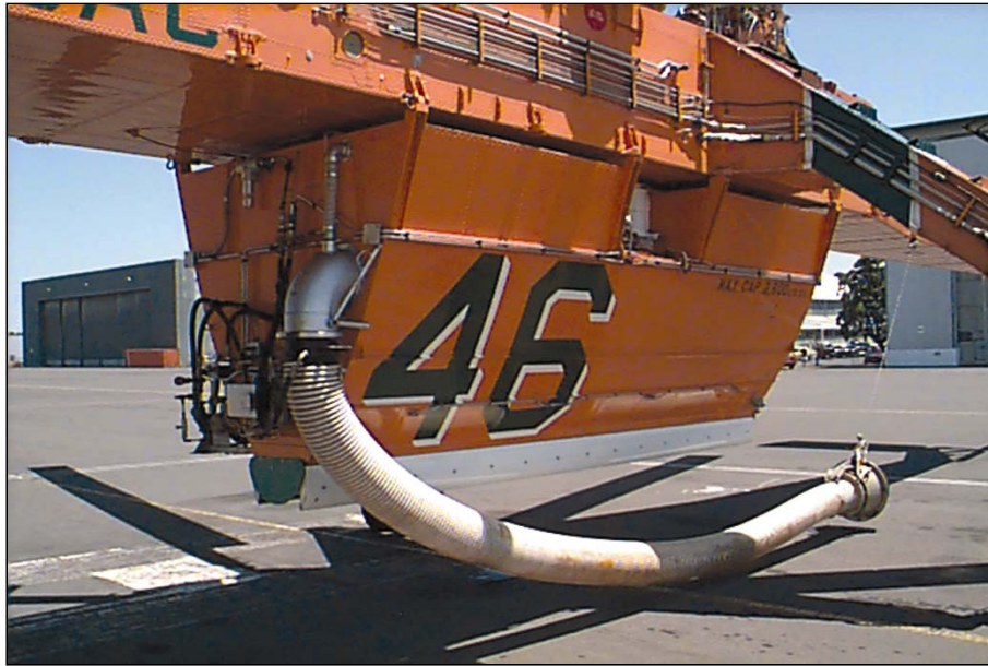
Figure 2 The 9500-litre firebombing tank under the Aircrane's fuselage
