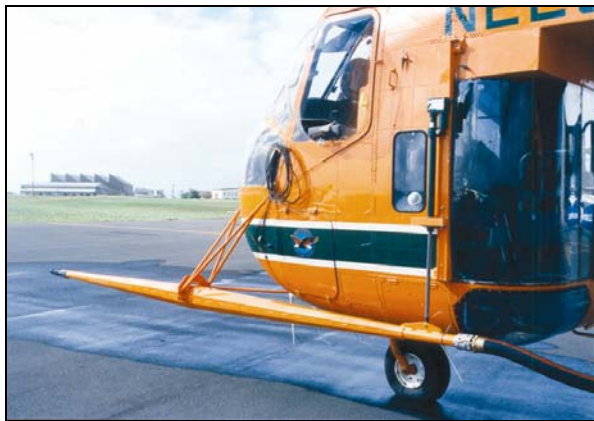
Figure 5 Water cannon fitted to the Aircrane
