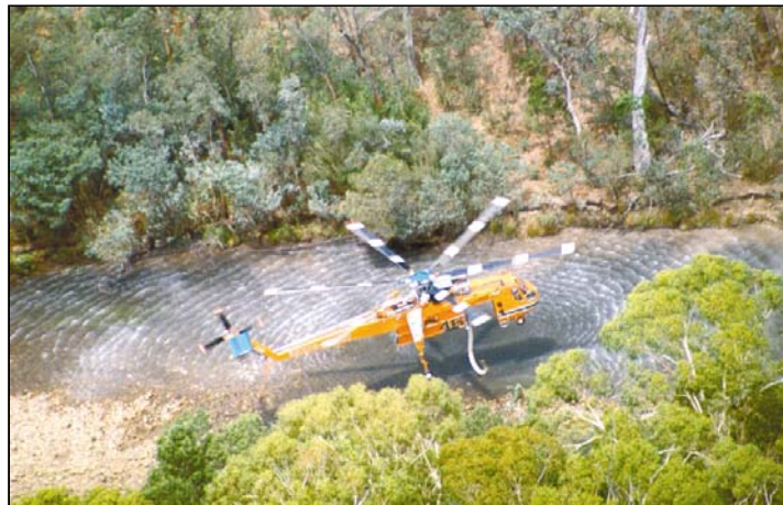
Figure 12 A minimum clearance of 70 metres diameter is required (Wonnangatta River – Caledonia fire 1998)
