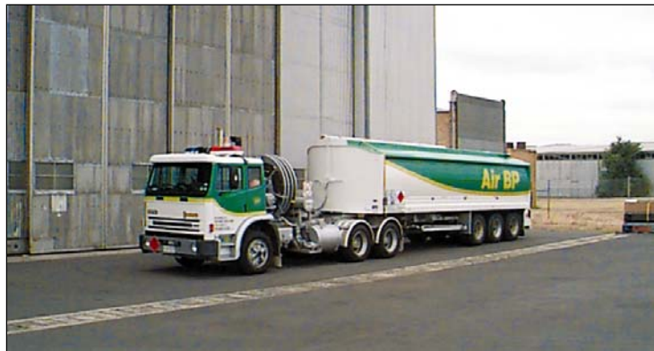
Figure 13 The 30 000-litre pressurised refuelling tanker
