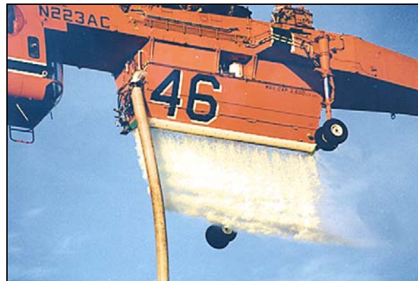
Figure 7 The long, narrow drop pattern from the Aircrane firebombing tank
