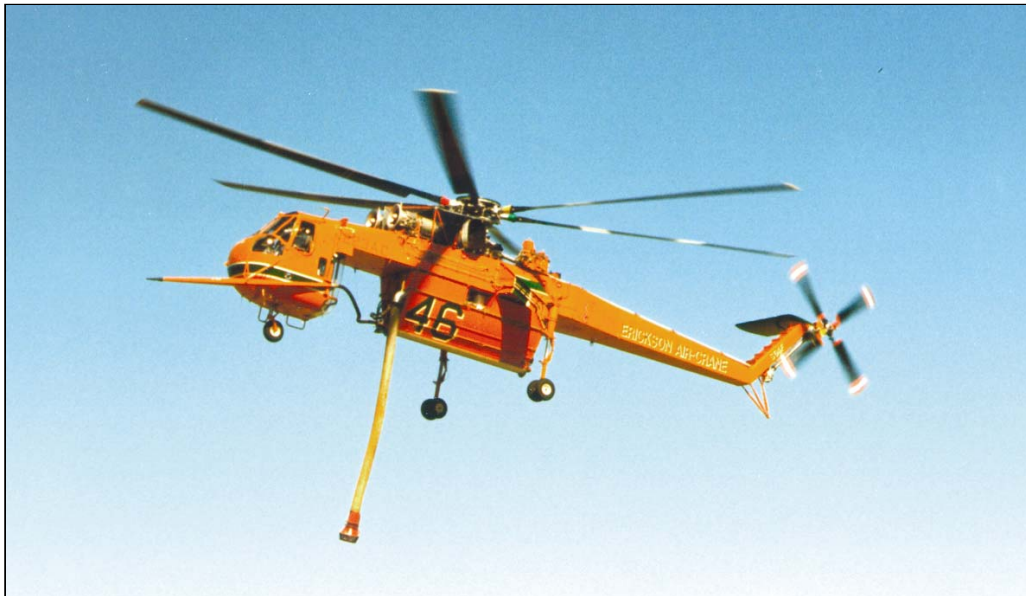
Figure 1 The S-64F Aircrane Helitanker
