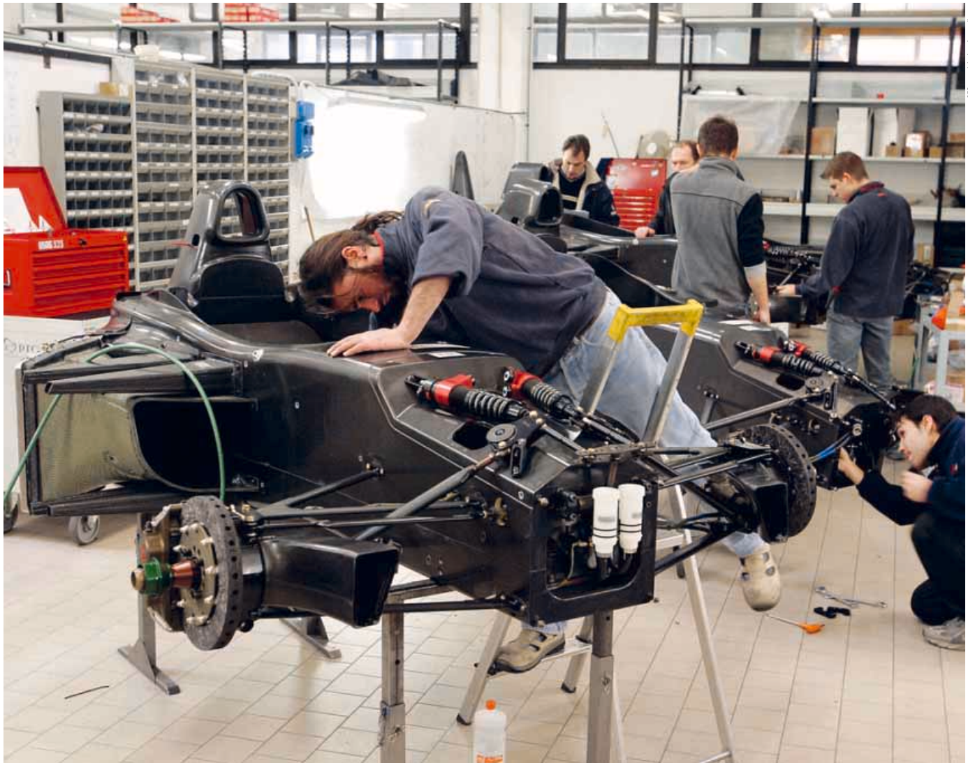
Using 3D CAD means the process from initial design, through detail design to production of final assemblies, such as these Dallara GP2 chassis, is accelerated
