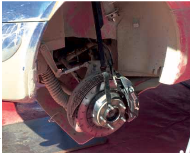
One step ahead – Citroën's extra brake cooling proved advantageous in Mexico
