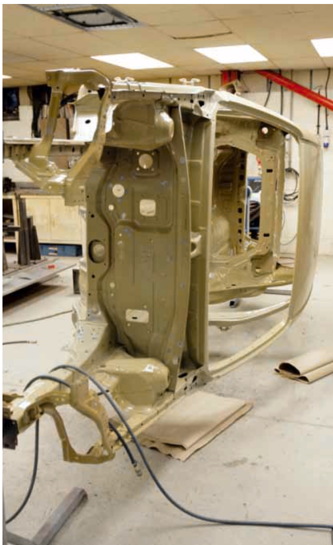
Lacetti 'shell has high inherent stiffness, making it an ideal for a WTC car
