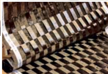
The difference is in the weave – main picture shows Oxeon’s innovative 50x50mm wide strand weave, while inset picture above shows an alternative 20x50mm weave
