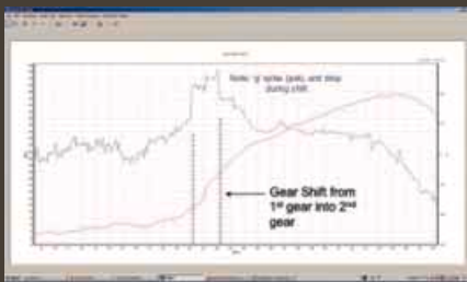
Rolls Royce Silver Spirit three-speed auto During the change the g trace exhibits a sharp spike produced by a surge from the engine inertia
