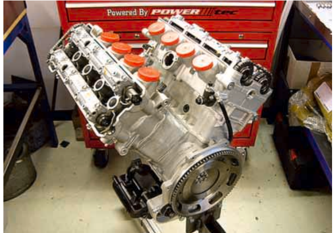
Features such as its in-line twin oil and water pumps, four-pump scavenge system and twin rotating balance shafts were all designed in SolidWorks
