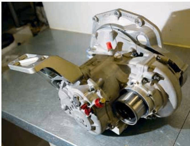
A specially-designed bellhousing is used to mate the gearbox and engine
