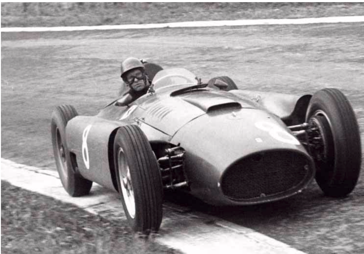
Pontoon fuel tanks, designed to keep the weight of the fuel load amidships was exploited on the Lancia-Ferrari D50
