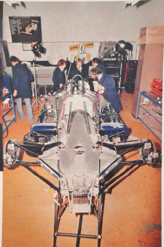
The Tolemans are powered by a turbocharged version of Brian Hart's successful 420R Formula 2 engine. The four cylinder, single turbo unit gives 525 bhp. Hart (opposite) is a former driver himself. He raced in actor Peter Sellers's F3 team, and then moved on to the wooden F2 Protos. His own engine designs later powered Mike Hailwood's Matchbox Surtees to victory in the European F2 championship of 1972. Last year Hart again won the F2 championship, his engines powering Henton's Toleman to victory and Warwick's similar car to runner-up position. Although Rory Byrne had provided space at the rear of the F1 Toleman for different intercooling solutions, he has since redesigned the back end of the car to accommodate more intercooling.
