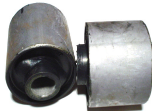
TOYOTONA BUJE TENS. TRAS. GRANDE COD. B81005 C487066030 18x55x60
