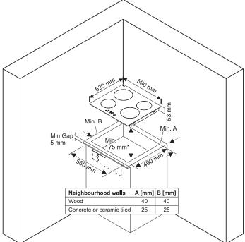
\*: In case of installation over a built-in oven, distance should be min. 10 mm.
