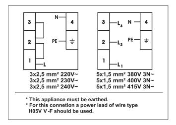
For the induction hob, the cable must be H05VV-F 3X2,5 mm²/60227 IEC 53 ••. You will find the connection diagram shown on the bottom of your appliance.
