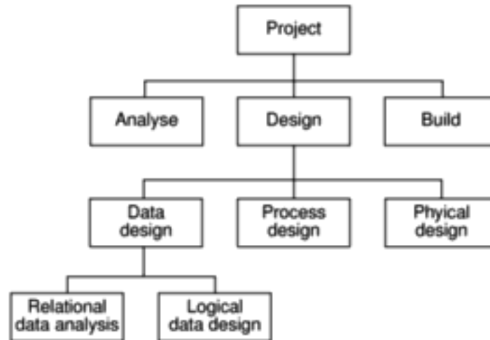
Figure 6.2 A fragment of an activity-based Work Breakdown Structure.
