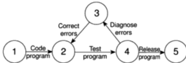
Figure 6.10 A loop represents an impossible sequence.
