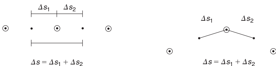
Figure 11-3 Illustrating calculation of \Delta s when path is sharply curved at the right, as opposed to the case when the path is essentially straight, as shown at the left.
