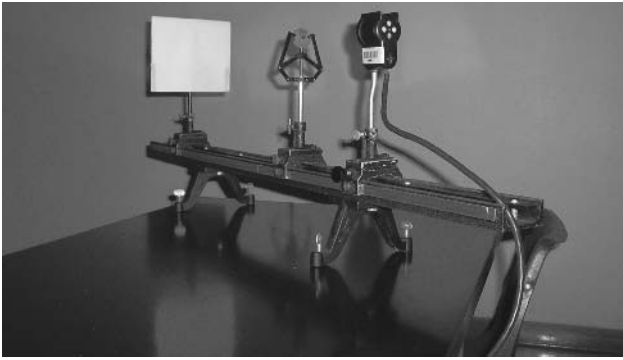
Figure 41-2 Optical bench with object, lens, and screen on which a real image is formed.
