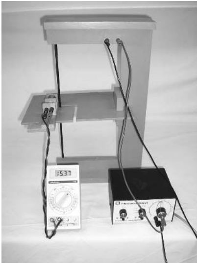
Figure 35-5 Homemade long wire apparatus with inductor coil in position.
