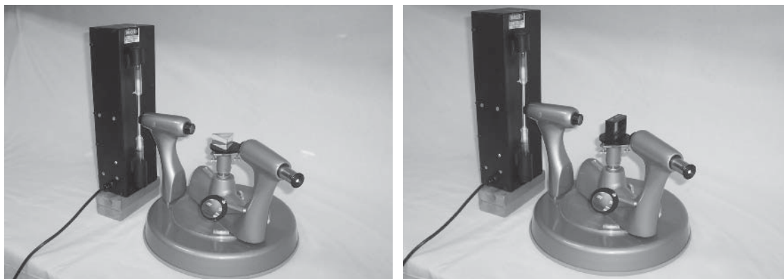
Figure 43-1 Spectrometer that can be used with a prism or with a diffraction grating.
