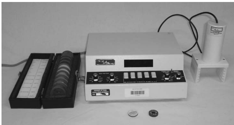
Figure 47-1 Geiger counter and set of standard absorbers described in procedure.
