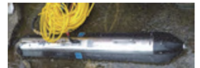
Side-scan sonar used in the experiment
