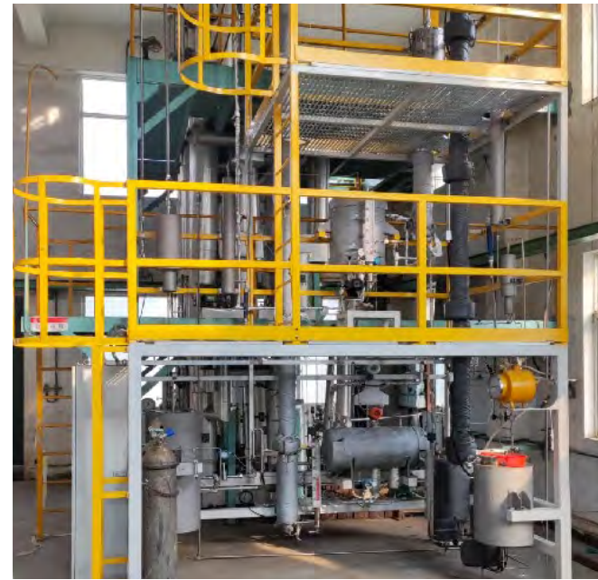
Figure 2: 3Nm 3 /h phase change absorber enlarge test
