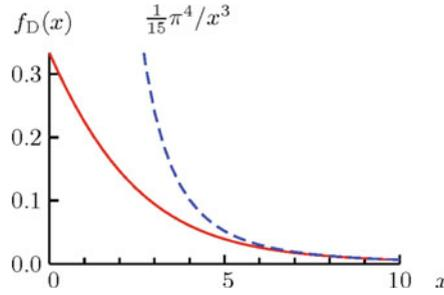
**Fig. 6.25** Debye function (continuous red curve) and its approximation  $\frac{1}{15}\pi^4/x^3$  (dashed blue curve)
