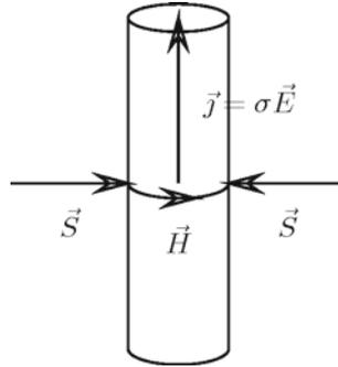
**Fig. 3.16** Interpretation of the Poynting vector  $\mathbf{S}$  for a stationary current along a wire of length  $l$  with radius  $R$ . Here  $\mathbf{S}$  flows from the outside through the curved surface  $A$  and, because  $E = U/l$  and  $H = I/(2\pi R)$ , it has the absolute value  $S = UI/A$  there. The heat power  $UI$  generated inside then flows out through the curved surface, while the current flows through the faces
