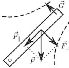
**Fig. 2.2** Lever law. The rigid lever transmits all those forces to the axle bearing (*open circle*) which do not have an angular momentum with respect to the axis—they are canceled by forces of constraint, here by  $\mathbf{F}_{\parallel}$ . Equilibrium prevails, if the torque due to the force  $\mathbf{F}$  and the counter-force  $\mathbf{G}$  cancel each other, as indicated by the two hyperbola branches
