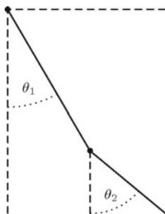
**Fig. 2.38** Double pendulum made from rods of mass  $m_1$  and  $m_2$  and with moments of inertia  $I_1$  and  $I_2$  with respect to the hinges ( $\bullet$ ), which are separated by a distance  $l$ . The distances of the centers of mass of the rods from the hinges are  $s_1$  and  $s_2$ , respectively
