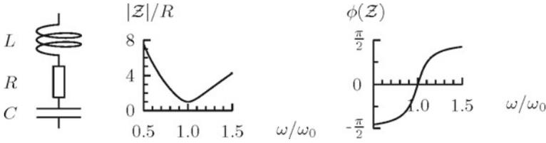
**Fig. 3.17** Absorption circuit. Resonance for  $\omega_0 = 1/\sqrt{LC}$ . Here,  $\omega_0 L = 5R$
