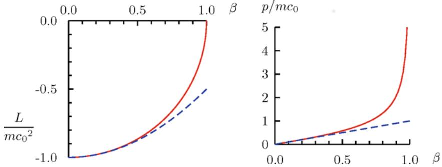
**Fig. 3.29** Lagrange function and momentum of free particles as a function of  $\beta = v/c_0$ : non-relativistic (*dashed blue*) and relativistic (*continuous red*)
