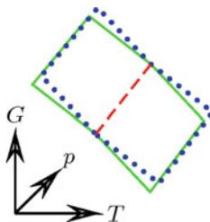
**Fig. 6.17** For first order phase transitions, the first derivative of the free enthalpy  $G(T, p)$  makes a jump, here indicated by the *dashed red line*. The structure indicated by the *dotted blue lines* would have higher  $G$  than the stable phase (*continuous green lines*). Here  $\partial G/\partial T = -S < 0$  and  $\partial G/\partial p = V > 0$  always hold
