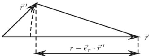
**Fig. 3.30** The approximation  $|\mathbf{r} - \mathbf{r}'| \approx r - \mathbf{e}_r \cdot \mathbf{r}'$  valid for  $r \gg r'$  follows by calculation (using a series expansion) as well as geometrically. The circular radius  $|\mathbf{r} - \mathbf{r}'|$  and the double-headed arrow are nearly equally long
