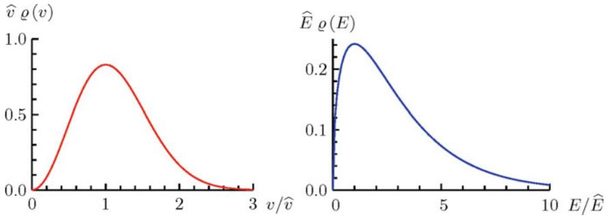
**Fig. 6.11** Maxwell distributions.  $\rho(v)$  (left),  $\rho(E)$  (right) in suitable temperature-independent units:  $\hat{v} = \sqrt{2kT/m}$  and  $\hat{E} = \frac{1}{2} kT$
