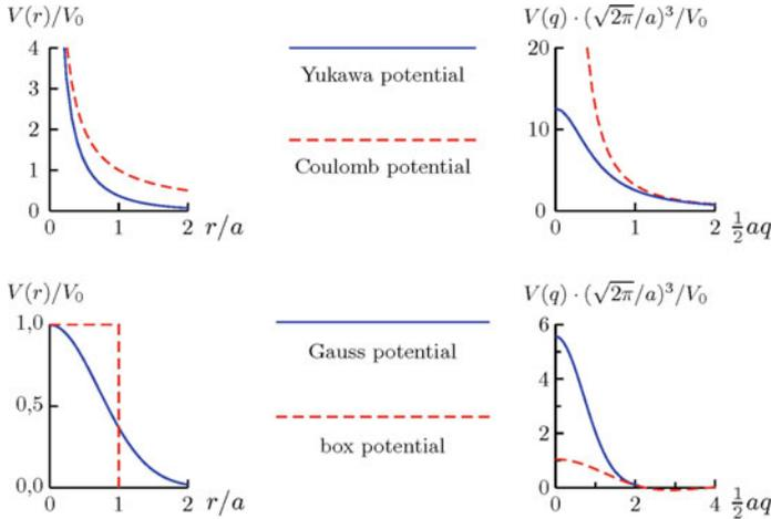
**Fig. 5.4** Fourier transforms of several isotropic potentials. *Top:* Yukawa and Coulomb potentials. *Bottom:* Gauss and box potentials. With  $\frac{1}{2}q = k \sin \frac{1}{2}\theta$ ,  $V(q)$  can be used in the Born approximation  $T(q) \approx V(q)$  for the differential scattering cross-section, as will be shown
