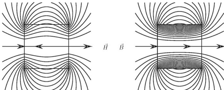
**Fig. 3.10** Field lines of a permanent homogeneous magnetized cylinder. *Left:*  $\mathbf{H}$  field. *Right:*  $\mathbf{B}$  field. Except for the edges, the flux through the surface increases by one unit from line to line. The *right-hand figure* applies also to the  $\mathbf{H}$  and  $\mathbf{B}$  field of a current-carrying coil
