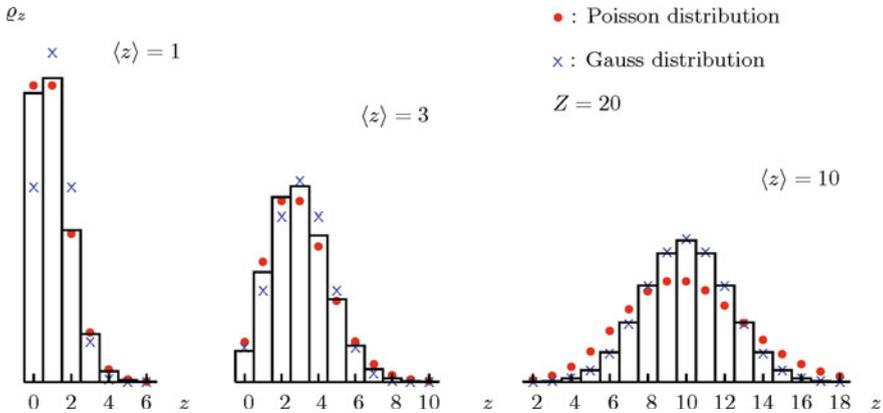
**Fig. 6.1** Binomial distributions (Bernoulli distributions), represented by bars, with 20 possibilities and the mean values  $\langle z \rangle \in \{1, 3, 10\}$ . For comparison, we also show the values for the associated Poisson and Gauss distributions
