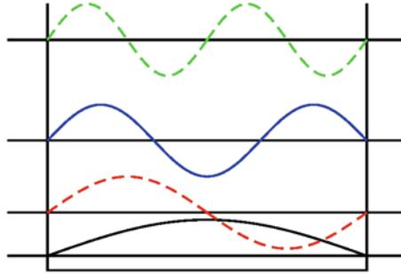
**Fig. 4.12** Energy eigenvalues and eigenfunctions of a box potential with infinitely high walls. The figure shows the potential and also the eigenvalues as *horizontal lines*. Each of these lines serves as an axis for the associated eigenfunction, where functions with even  $n$  are plotted with *continuous lines*, and those with odd  $n$  as *dashed lines*
