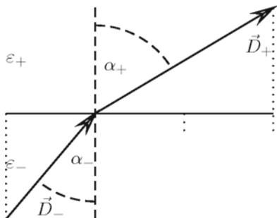
**Fig. 3.6** Diffraction of the electric field entering into an insulator of higher permittivity (here  $\epsilon_+ = 2\epsilon_-$ ). The force lines become diffracted away from the normal. In contrast, according to the optical *diffraction law* (see p. 220) the rays become diffracted towards the normal for  $n_+ > n_-$  and, instead of  $\tan \alpha$ , we have in that case  $\sin \alpha$
