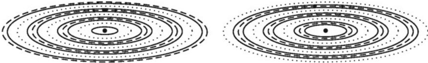
**Fig. 3.33** Magnetic field lines of the Hertz dipole at the same times as in Fig. 3.32, here in an inclined view of the central plane. At the *dotted lines*,  $B$  is extremal again, while at the *dashed lines*, the field direction is reversed
