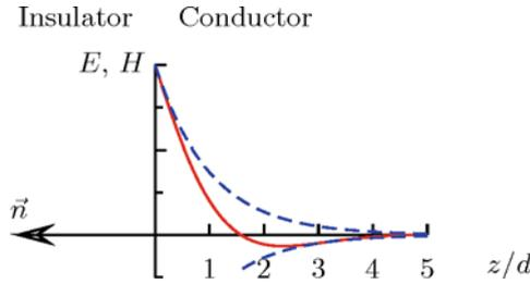
**Fig. 3.22** Repulsion of the current. Decay of the alternating fields in the interior of a conductor—*dashed lines* show their amplitude—here for  $\sigma \gg \varepsilon\omega$  and hence  $\alpha \approx \beta$ . (When  $\sigma/\varepsilon\omega < \infty$ , there is also a normal component of the magnetic field and a tangential component of the electric field)
