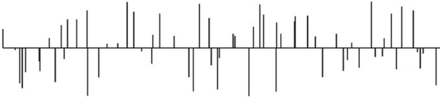
**Fig. 6.9** Stochastic force as a function of time. This acts irregularly in time, strength, and direction (only one component is shown here)
