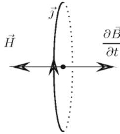
**Fig. 3.15** Lenz's rule. The time-dependence of the magnetic field  $\partial \mathbf{B} / \partial t = -\nabla \times \mathbf{E}$  induces a current density  $\mathbf{j} = \sigma \mathbf{E}$  in the conductor loop. This current is accompanied by a magnetic field curl density  $\nabla \times \mathbf{H} = \mathbf{j}$  such that, on the plane of the loop,  $\mathbf{H}$  and  $\partial \mathbf{B} / \partial t$  are oriented in opposite directions
