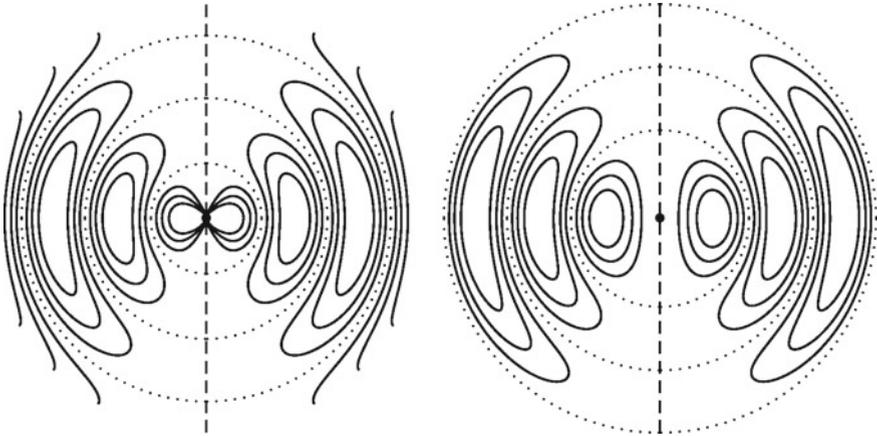
**Fig. 3.32** Electric field lines of the Hertz dipole at two times. At the circles (*dotted lines*), the curl densities reverse  $\odot \leftrightarrow \ominus$ , and so also does  $\partial \mathbf{B} / \partial t$ , implying that  $B$  is extremal there
