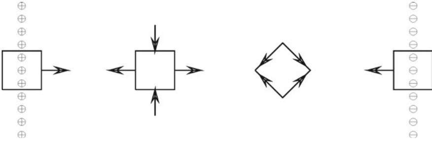
**Fig. 3.7** Visualization of the Maxwell stress tensor for a homogeneous electric field (the field strength points from the  $\oplus$  to the  $\ominus$  charges). Shown are the surface tensions on four cubes—depending on their charge, the forces on opposite faces either cancel or supply the expected force (see Problems 3.21–3.22)
