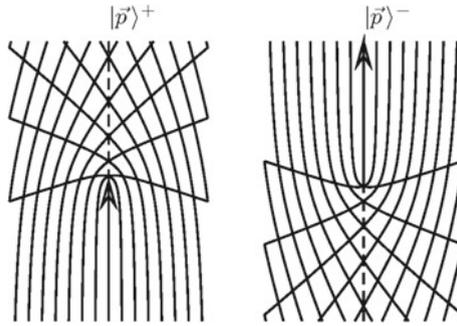
**Fig. 5.5** The scattering states  $|\mathbf{p}\rangle^\pm$  (momentum upwards) with an attractive Coulomb potential, represented by the classical orbital curves (calculated according to Sect. 2.1.6). From orbit to orbit, the collision parameter changes each by one unit. Quantum-mechanically, sharp orbits are not allowed—this is to be noted particularly for the straight orbit through the center
