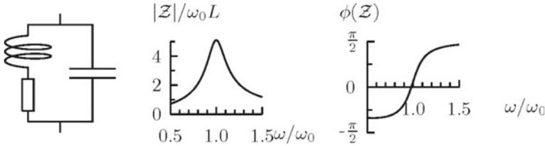
**Fig. 3.18** Trap circuit. Resonance occurs for  $\sqrt{\omega_0^2 - (R/L)^2}$ . Note that here  $\omega_0 L = 5R$
