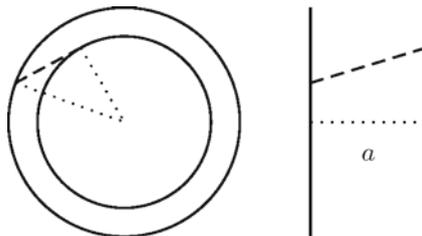
**Fig. 3.13** Top and side view of two coaxial current loops (*continuous lines*) at the distance  $a$ . The line  $|\mathbf{r} - \mathbf{r}'|$  connecting two points is shown by a *dashed line*. It can be calculated with the help of the *dotted lines* (radii  $R$  and  $R'$ )
