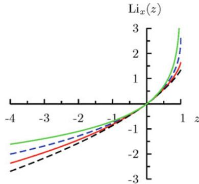
**Fig. 6.23** The logarithm  $\text{Li}_x(z) = \sum_{n=1}^{\infty} \frac{z^n}{n^x}$  for  $|z| < 1$ , *continuous* for  $x = 1$  (green) and  $2$  (red), *dashed* for  $x = \frac{3}{2}$  (blue) and  $\frac{5}{2}$  (black). The name stems from  $\text{Li}_1(z) = -\ln(1 - z)$ . Then  $\text{Li}_2(z)$  is also called the *dilogarithm*. Furthermore,  $\text{Li}_x(1) = \zeta(x)$  and  $\frac{d\text{Li}_x}{dz} = \frac{\text{Li}_{x-1}(z)}{z}$  (also for  $|z| \geq 1$ )
