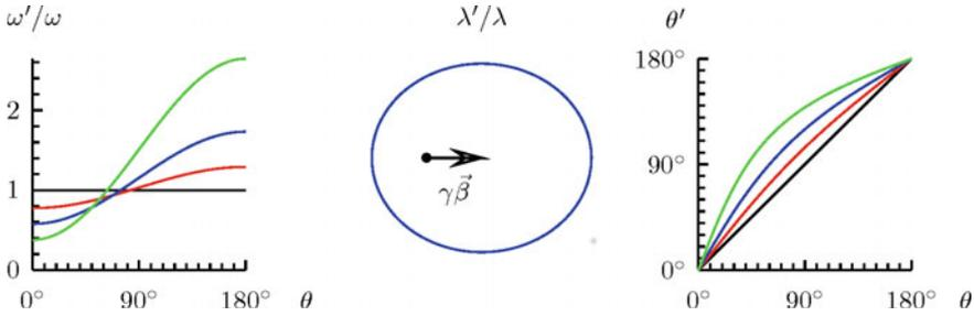
**Fig. 3.26** Angular dependence of the frequency, wavelength, and deviation. In the *left and right figures*, straight lines refer to  $\beta = 0$  (black), the curves to  $\beta = \frac{1}{4}$  (red),  $\frac{1}{2}$  (blue), and  $\frac{3}{4}$  (green). The *middle picture* shows the ratio of the wavelengths  $\lambda'/\lambda$  in a polar diagram, namely the focal representation of an ellipse with semi-axes  $\gamma$  and 1, and hence eccentricity  $\beta$  (here 1/2). See also Fig. 3.31
