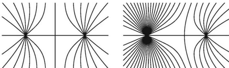
**Fig. 3.2** Field lines of two like charges—the ratio of the charges *on the left* is 1:1 and *on the right* 3:1—with their saddle point between the two charges
