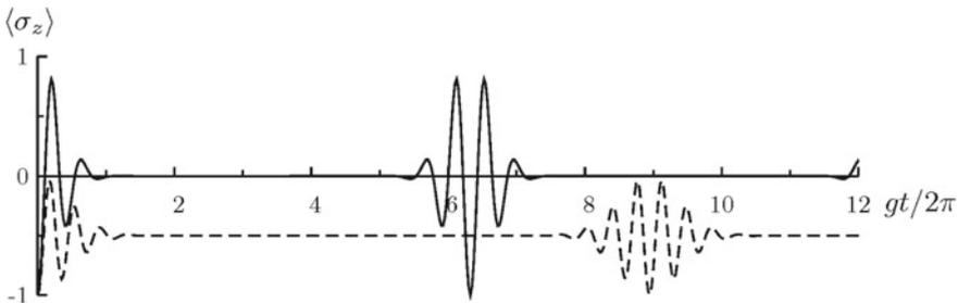
**Fig. 5.19** Absence and return of the excitation of an atom in a light field described by a Glauber state. Initially,  $|\alpha|^2 = 10$  and the atom was in the ground state. *Continuous curve*: resonance. *Dashed curve*: Detuning  $\Delta = |\alpha g|$ . Here  $\langle \sigma_z \rangle = 0$  indicates that on average there are equally many atoms in excited states as in the ground state
