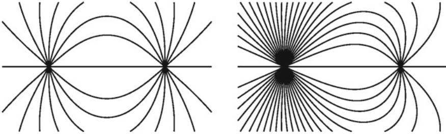
**Fig. 3.3** Field lines of two unlike charges—ratio of the charges again 1:1 and 3:1 on the *left* and *right*, respectively
