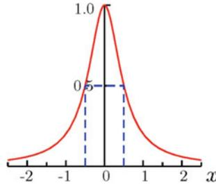
**Fig. 5.6** Lorentz curve  $\frac{1}{4}/(x^2 + \frac{1}{4})$  (continuous red), line shape of a scattering resonance about the resonance energy  $E_R$  with half-width  $\Gamma$ , where  $x = (E - E_R)/\Gamma$ . The curve has half the maximum value at two points which have the distance of the half-width (dashed blue). For this distribution,  $\Delta E = \infty$  and the associated average lifetime is  $\hbar/\Gamma$
