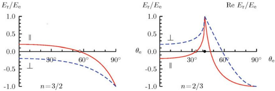
**Fig. 3.21** Fresnel’s equations for the transition from air to glass ( $n = 3/2$ ) and back. Brewster angle  $\circ$ . Limiting angle for total reflection  $\bullet$  (for larger angles, only  $\text{Re}E_r/E_e$  is shown)
