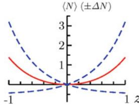
**Fig. 5.16** Influence of the quench parameter  $z$  on the particle number (continuous red) and its uncertainty  $\Delta N = \sqrt{|u\beta - v\beta^*|^2 + u^2v^2}$  (dashed blue), here shown for the quenched vacuum. The average particle number is in fact then as small as possible for a given  $z$ , but greater than zero for  $z \neq 0$
