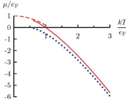
**Fig. 6.22** The chemical potential of an ideal monatomic Fermi gas as a function of temperature, relative to the Fermi energy  $\epsilon_F = (9\pi/16)^{1/3} kT_0$  with  $kT_0$  from Fig. 6.19. The *continuous red curve* corresponds to the high-temperature expansion, the *dashed magenta curve* to the low-temperature expansion, and the *dotted blue curve* to a Bose gas (see Fig. 6.29 for Bose–Einstein condensation)
