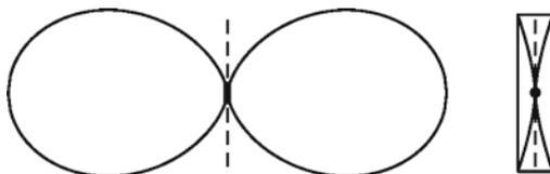
**Fig. 3.4** Field lines of a dipole pointing along the *dashed symmetry axis*. *Right*: The field in the middle is magnified eight times. All other field lines are similar to the ones shown here, because point-like sources do not provide a length scale (see Problem 3.14)
