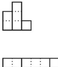
**Fig. 6.3** Information measure for  $\{\rho_1 = \frac{1}{3}, \rho_2 = \frac{1}{2}, \rho_3 = \frac{1}{6}\}$ . This is indicated here by the upper probability distribution. The problem can be mapped onto  $Z' = 6$  equally probable cases, whence the steps turn into a single bar of equal area. With the additivity of the information measure, it then follows that  $\text{lb}6 = I_1 + \text{lb}2 = I_2 + \text{lb}3 = I_3 + \text{lb}1$  and hence  $I_z = -\text{lb}\rho_z$
