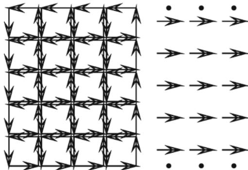
**Fig. 3.9** *Left:* A macroscopic current loop (in the  $y, z$ -plane) is divided into  $4 \times 5$  “microscopic” ones, each of which represents a magnetic moment. *Right:* A cuboid with three such planes with magnetic moments (*arrows*) is cut open (in the  $x, z$ -plane) and a current loop is associated with each one. The intersection points of the currents are indicated by the *black dots*
