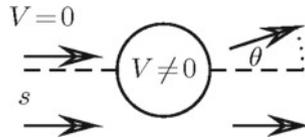
**Fig. 5.1** Scattering with scattering angle  $\theta$  (angle of deflection) and collision parameter  $s$  (see Fig. 2.6). If  $s$  is too large, there is no scattering force
