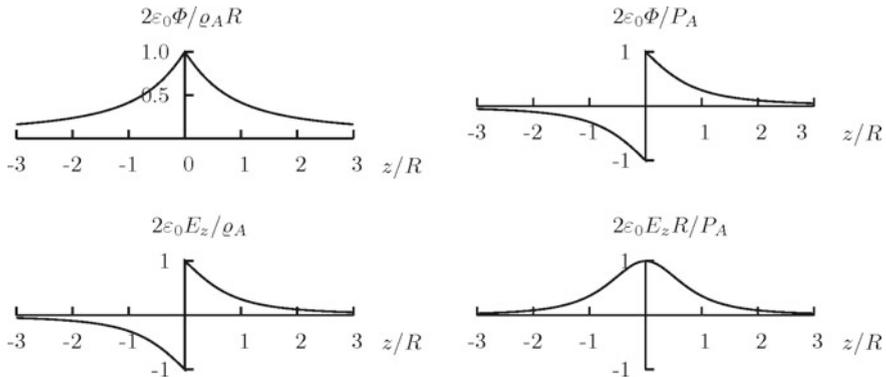
**Fig. 3.5** Potential (*upper*) and field strength (*lower*) along the axes of circular disks of radius  $R$ . The disk is loaded with monopole charge density  $\rho_A$  (*left*) or with dipole charge density  $P_A$  (*right*), where the potential discontinuity at the disk also leads to a delta function. The curve *lower right* diverges at  $z = 0$  (see Problems 3.18–3.19)
