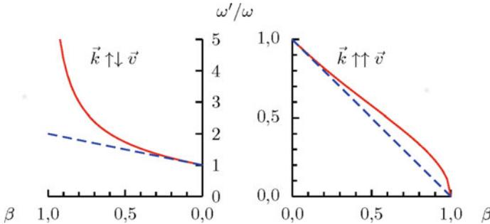
**Fig. 3.27** Doppler effect. A frequency depends on how fast the detector moves relative to the emitter. *Left:* Decreasing distance. *Right:* Increasing distance. The *linear Doppler effect* is indicated by the dashed line
