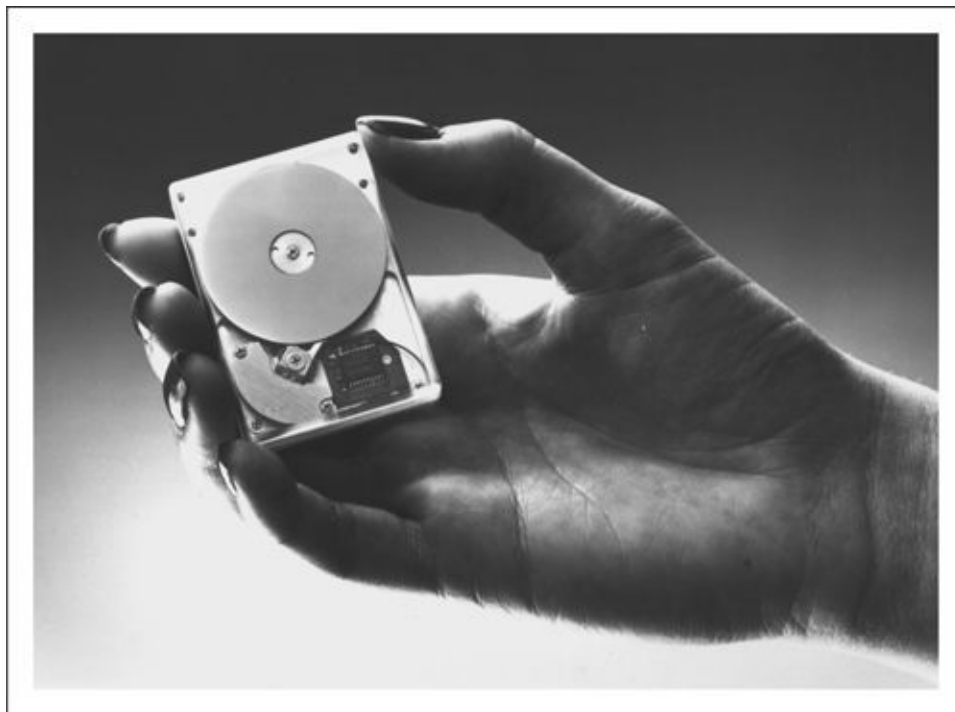
Figure 7.2 Hewlett-Packard's Kittyhawk Drive
