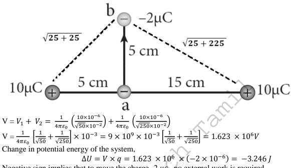
Negative sign implies that to move the charge  $-2 \mu c$ , no external work is required. System spends its stored energy to move the charge from te point a to b.
