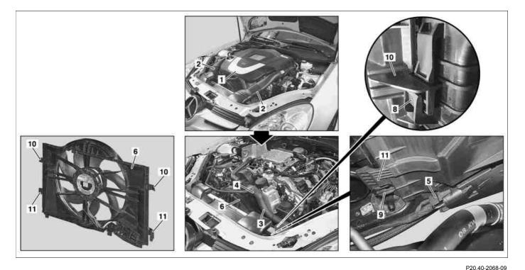
1 Front engine cover 2 Intake air duct Coolant hose
