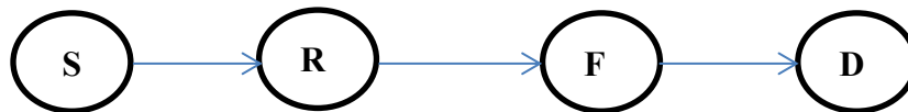
Figure 2. Example of sending a data packet from source node S to target D
