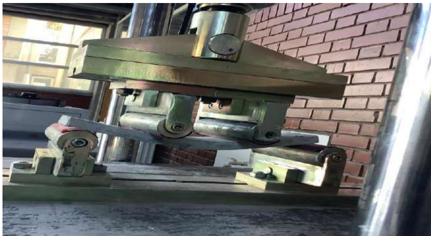
Figure 4. ECC deflected specimen
