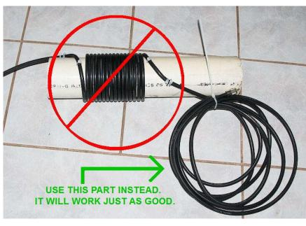
The truth is, the wrapped up extra coax to the bottom right of the pic would probably do the same and equally effective job as the perfectly wound coax on the PVC tubing. Believe it or not, it's true.
