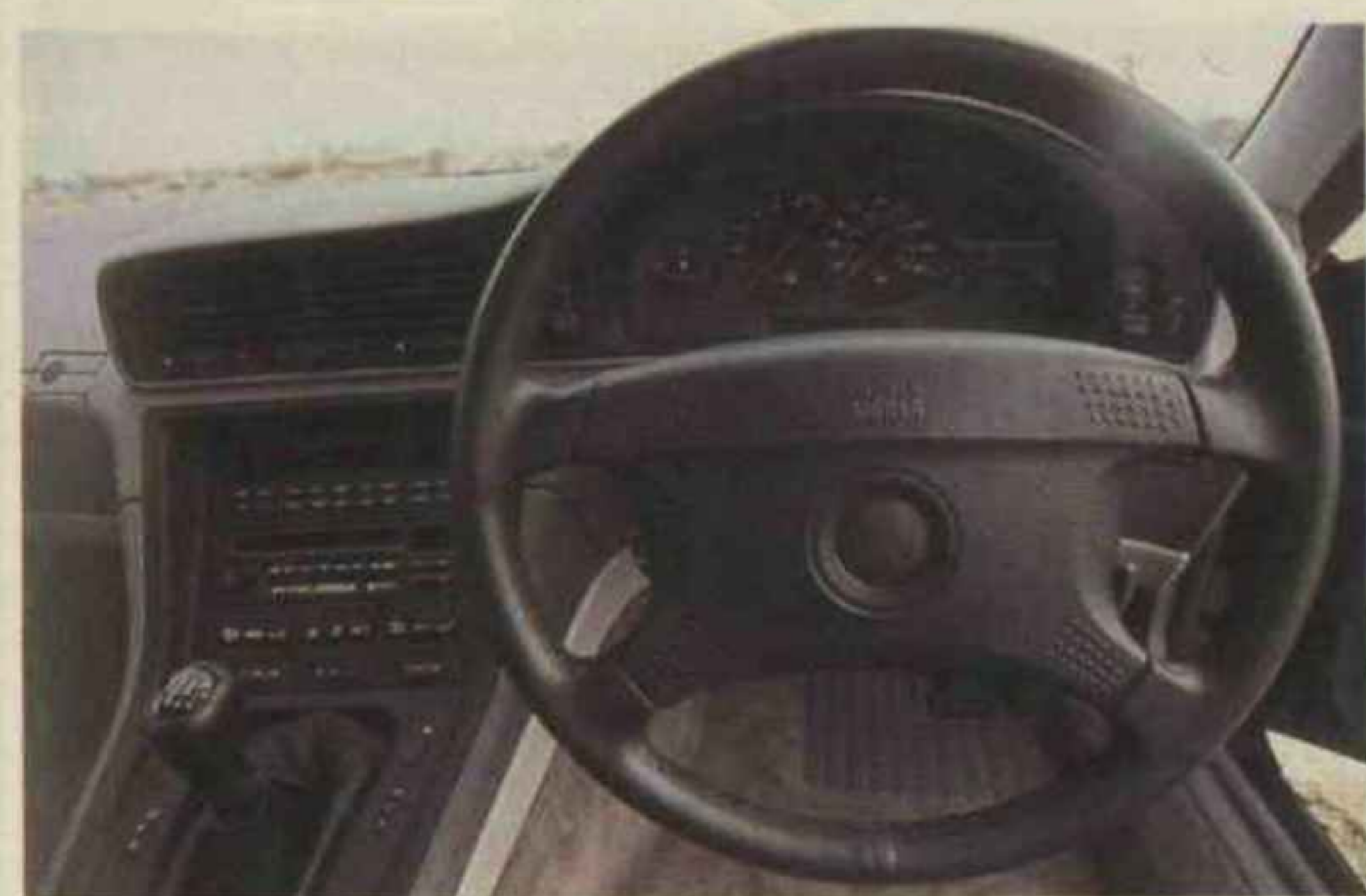
Airbag on steering wheel is compact. Instruments are not normal BMW style, but still clear. Switches for the 'clever bits' are on the centre console.
