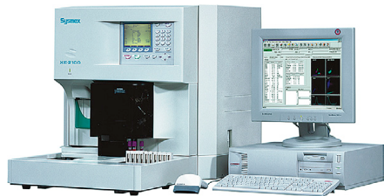
FIGURE 10-3 Hematology Automation; Sysmex XE-2100. (Courtesy Sysmex Inc., Mundelein, Ill.)
