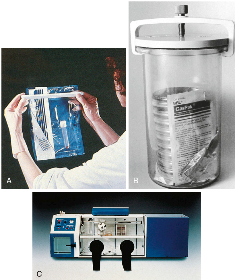
FIGURE 16-13 Anaerobic atmospheres can be created by using pouches, jars, or anaerobic chambers. A , Anaerobic pouch. B , Anaerobic jar. C , Anaerobic chamber. (A courtesy and copyright Becton Dickinson and Company; B from Forbes BA, Sahm DF, Weissfeld AS: Bailey and Scott's diagnostic microbiology , ed 12, St Louis, 2007, Mosby; C courtesy Anaerobe Systems, Morgan Hill, Calif.)
