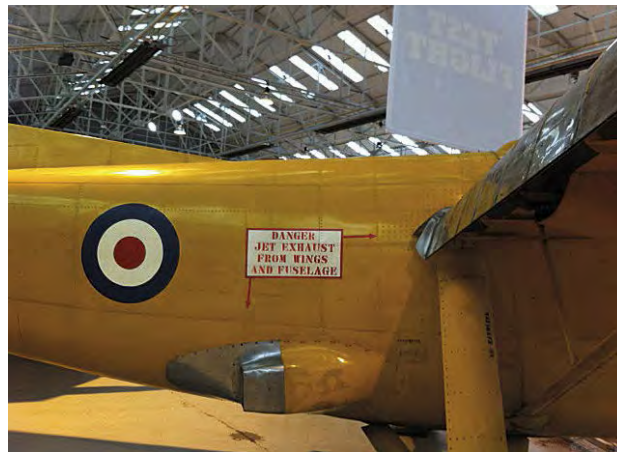
Hunting 126 aircraft of 1963 used blown flaps for low-speed lift, presaging in reverse F1's blown diffusers
