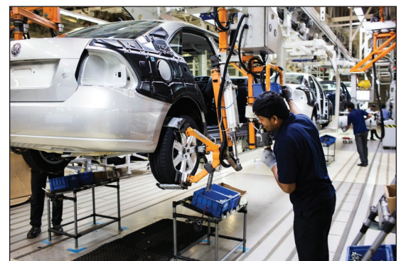
An employee uses a robotic arm to fit a wheel onto a Volkswagen AG Vento automobile on the production line at the Volkswagen India Pvt. plant in Chakan, Maharashtra, India.
