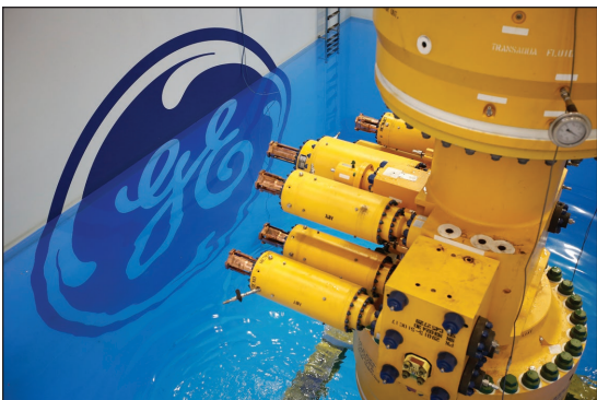
A subsea oil and gas tree is lowered into a testing pool at the General Electric Co. manufacturing plant in Montrose, United Kingdom.
