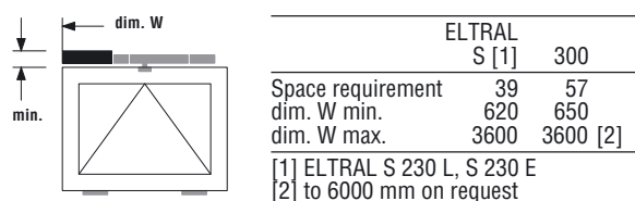
ELTRAL horizontal installation at the top
