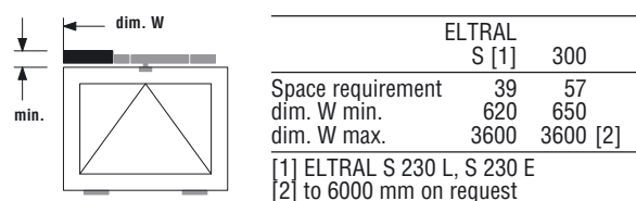
ELTRAL horizontal installation at the top
