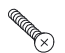
Inside/ outside operation Countersunk screw M 5 ST 50-54 9-13255-60-0-1 ST 55-59 9-13255-65-0-1 ST 60-64 9-13255-70-0-1 ST 65-69 9-13255-75-0-1 ST 70-74 9-13255-80-0-1 ST 75-80 9-13255-85-0-1
