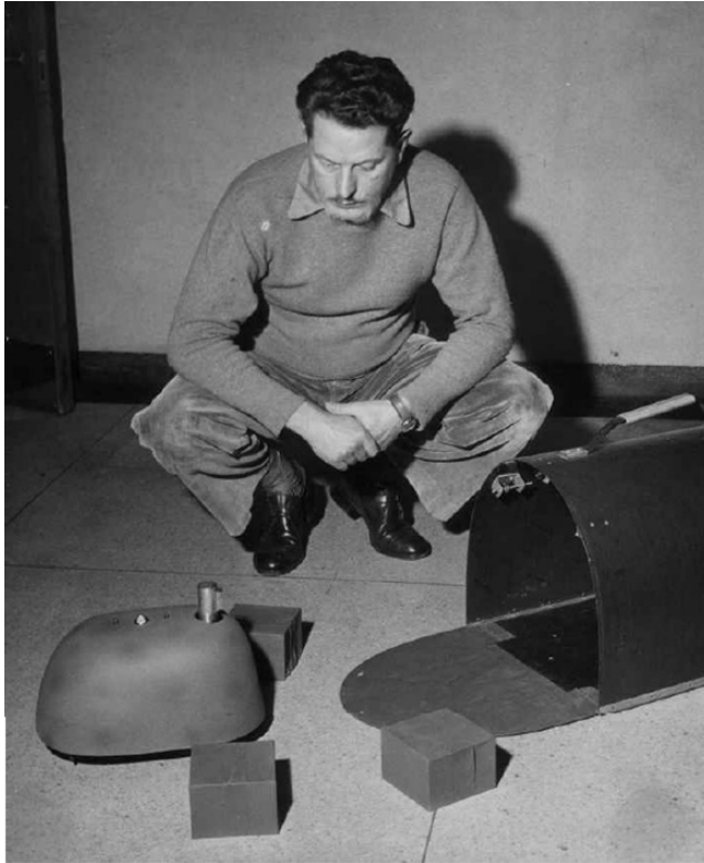
Figure 13.1 Grey Walter watches one of his tortoises push aside some wooden blocks on its way back to its recharging hutch. Circa 1952.
