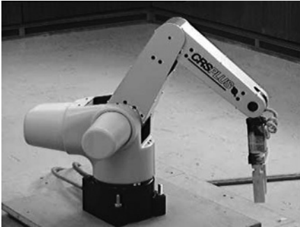
Figure 13.2 An articulated industrial robot arm. Arms vary in complexity with some involving more joints and a greater number of degrees of freedom.
