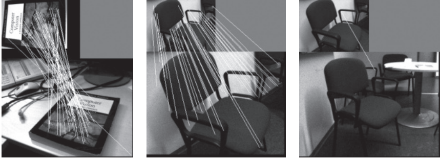
Figure 8.7 Matching result based on local descriptors (here SIFT; Lowe, 2004). First, salient points are computed on different scales. Then, the corresponding local descriptors are matched to a model database (given by the small image). Left is an ideal example of planar object that is highly textured. Middle and right examples show that the approach breaks down for less textured 3D objects if the perspective changes only slightly. In the right image only a single feature correspondence is found.
