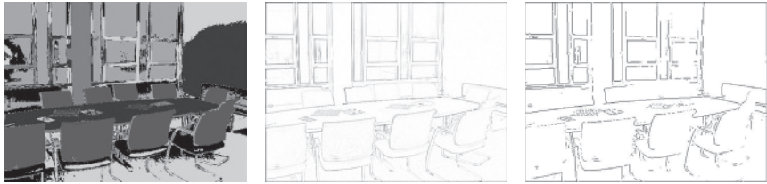
Figure 8.4 2D scene geometry. The left image shows a region segmentation based on a color clustering (shown with homogeneous gray values); in the middle a Difference of Gaussian (DoG) filter has been applied to the original image; the right image shows a contour segmentation based on the DoG image.
