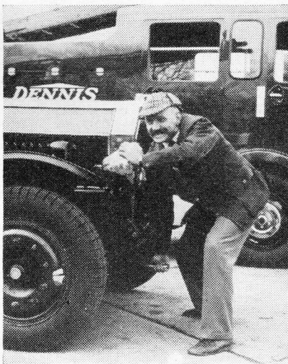
HEAVE HO! Bolster found starting the 9.4-litre four-cylinder engine quite a proposition, and was thankful there was not a real fire alarm!
