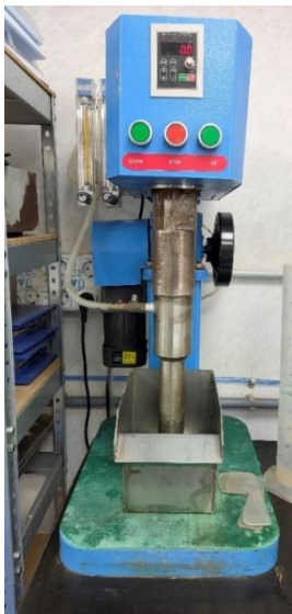
Figure 5. Flotation cell at AGQ.
