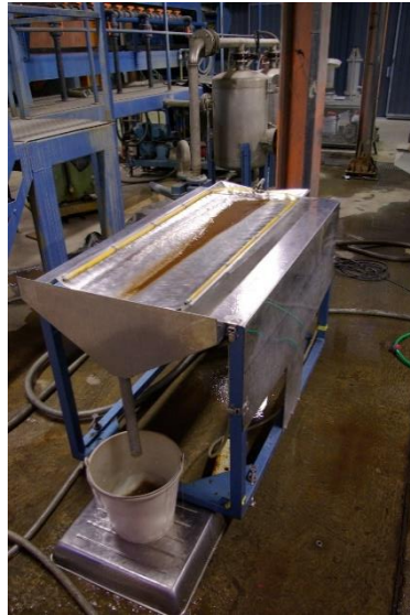
Figure 2. Mozley shaking table (@BRGM).
