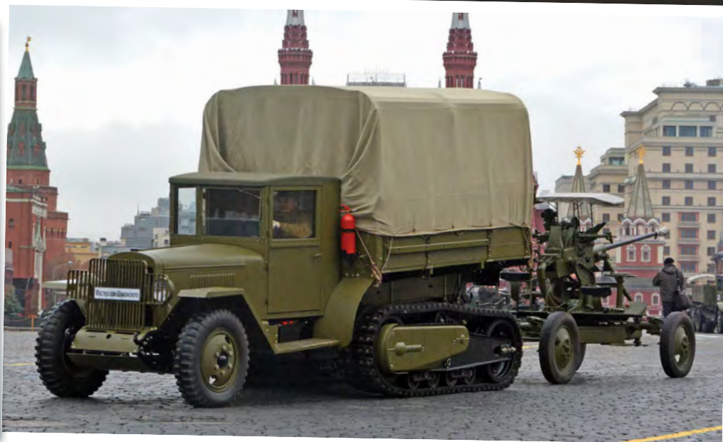
The ZiS-42 towing a 37mm M-1939 anti-aircraft gun through Red Square. (Andrey Aksenov)
