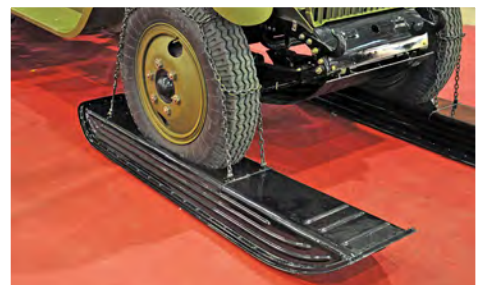
The ZiS-33's winter progress was aided by the use of pontoons on the front steering axle.
