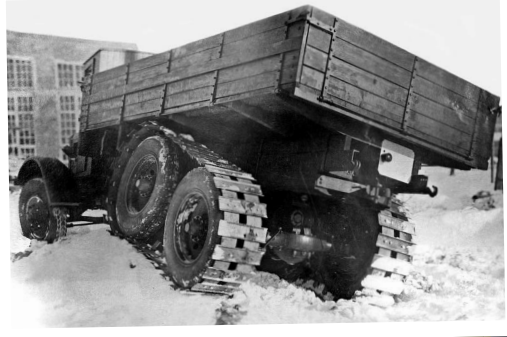
The alternative Russian option to half-tracks was the fitting of removable 'overall' tracks, mounted over the tandem rear wheels of conventional 6x4 trucks and BA-6 and BA-10 armoured cars.
