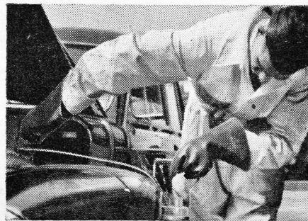
Taking a sample of the oil to be tested for radio-activity. It proved that BP Energol 'Visco-static' gives 80% less engine wear compared with conventional oils.
